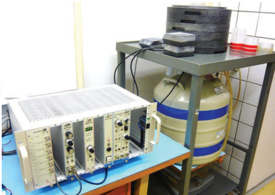
Figure 3. A high purity germanium detector (HPGe) set-up used in the passive method.
