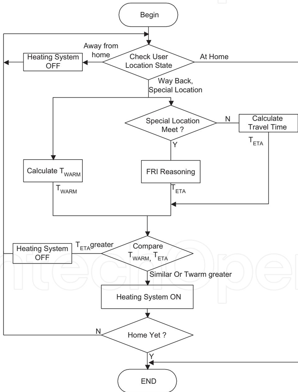
**Figure 5.** The flow chart of the heating controller [23].
