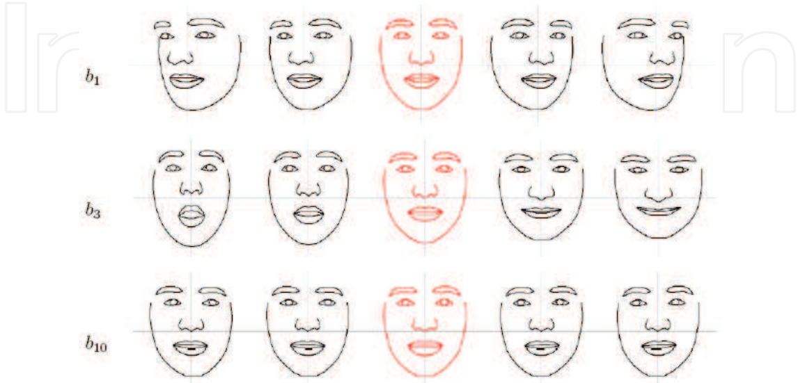
Figure 4. Deformation by change of just one parameter in each row. Topmost row: b_1 rotates the head. Middle row: b_3 opens the mouth. Lower-most row: b_{10} moves pupils in parallel
