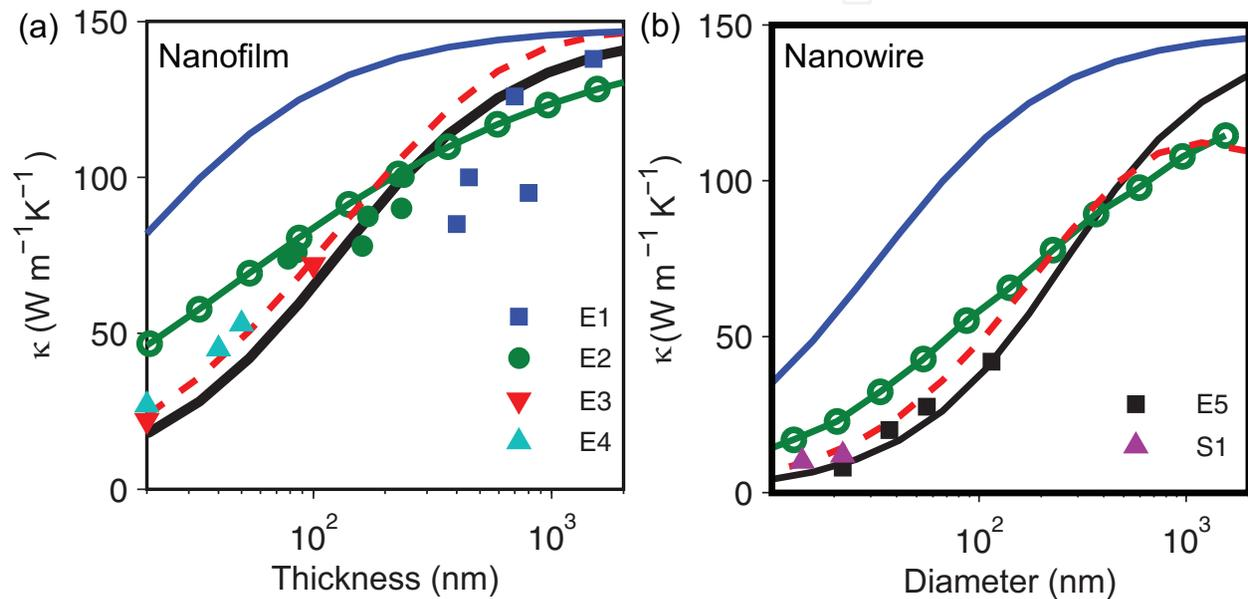
**Figure 2.** Effective in-plane thermal conductivities of single crystal Si nanosystems at room temperature. Bottom solid line: present model (Eq. (34)); top solid line: gray model [7]; solid and circle: McGaughey model [16]; dash line: Ma model [31]. (a) Nanofilm. Symbols E1–E4 are experimental results from Refs. [18–21]. (b) Nanowire. Square is experimental results from Ref. [25]. Triangle is numerical results from Refs. [41, 42].
