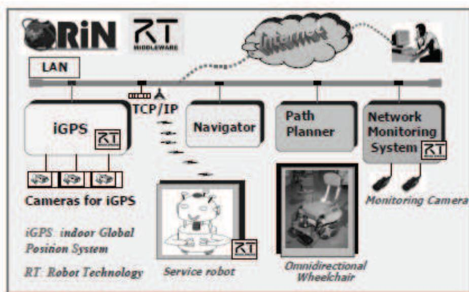
Fig. 4. Structure of the developed intelligent service robotic system.
