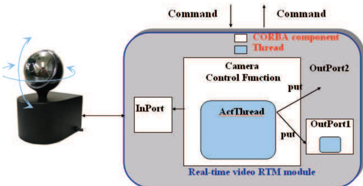
Fig. 10. Video/audio RT component developed based on RTM.
