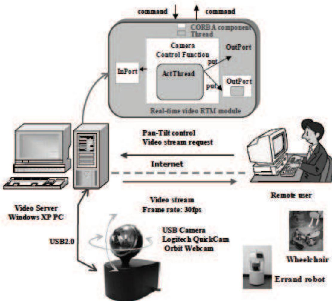
Fig. 12. Structure of RT video stream functional component.
