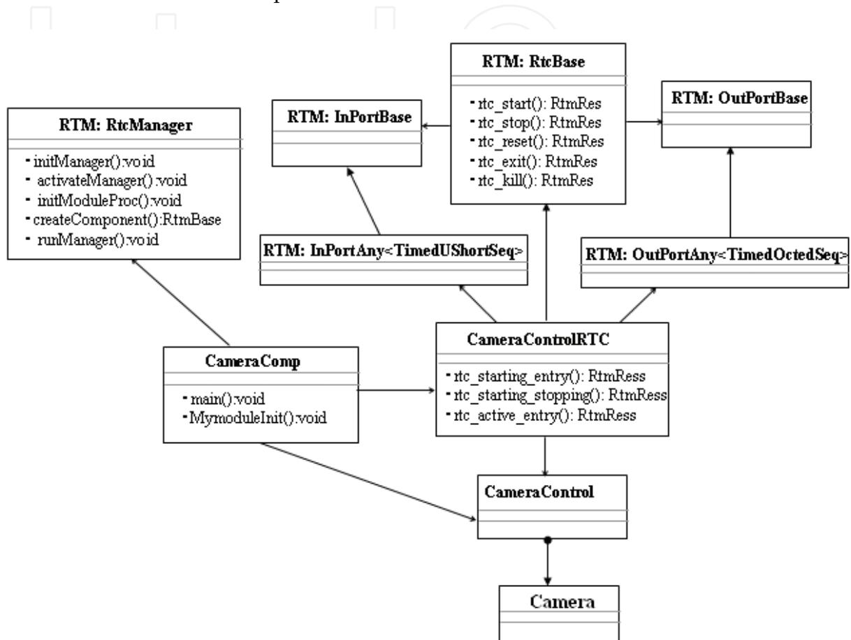
Fig. 11. Class structure of the developed RT component.
