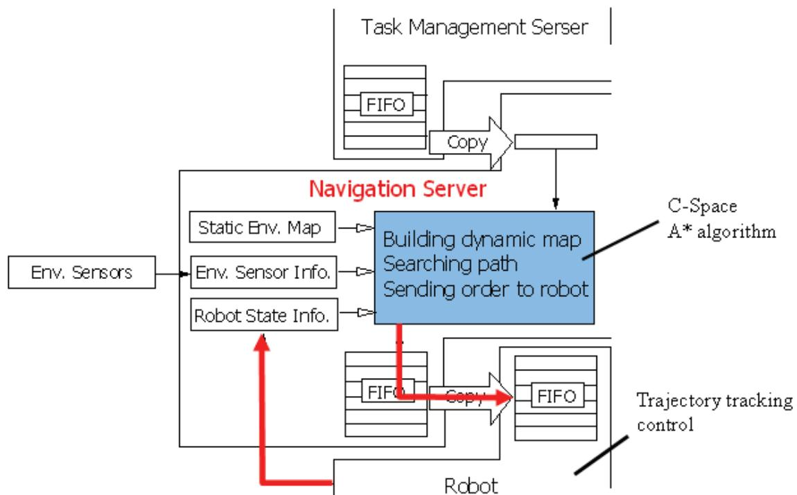
Fig. 8. Developed Errand mobile Robot navigation server.
