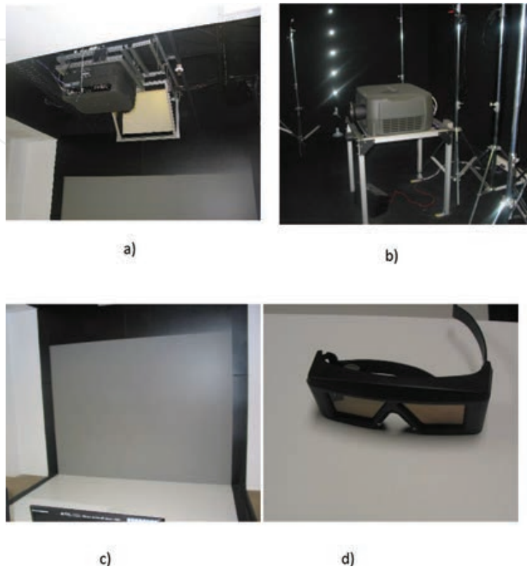
Figure 1. Elements of the virtual reality room. (a) and (b) Projectors, (c) 2 screens in an L shape, and (d) virtual reality glasses.
