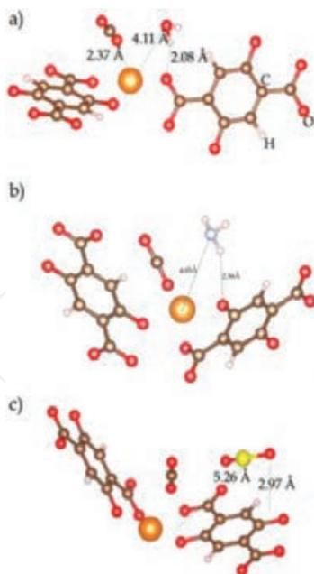
**Figure 13.** Adsorption configuration of the H<sub>2</sub>O (top), NH<sub>3</sub> (middle), SO<sub>2</sub> (bottom) molecule on Mg-MOF-74 fully loaded with CO<sub>2</sub> molecules at the metal centers. Red, brown, gray, blue, and orange spheres denote O, C, H, N, and Mg atoms, respectively. Parts of the MOF have been removed for visualization purposes. Reprinted with permission from [31]. Copyright (2015) American Chemical Society.
