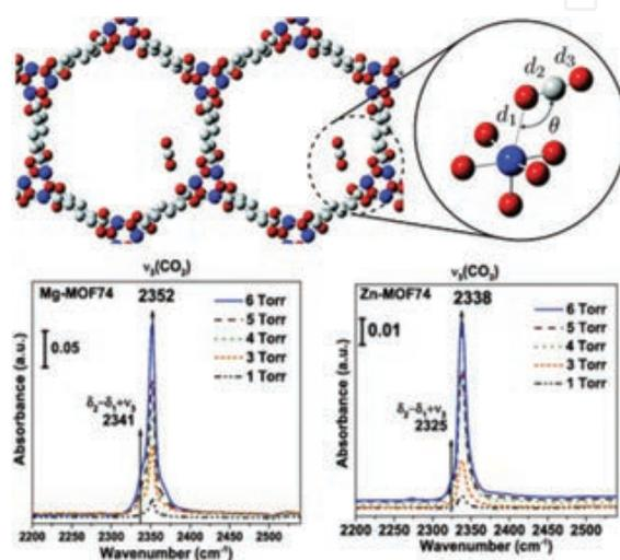
**Figure 2.** (Top) Illustration of CO<sub>2</sub> adsorbed in Zn, Mg-MOF-74. (Bottom) IR absorption spectra of CO<sub>2</sub> adsorbed into Mg-MOF-74 (bottom left) and Zn-MOF-74 (bottom right) at changing CO<sub>2</sub> pressure (1–6 Torr). Adapted with permission from [4]. Copyrighted by the American Physical Society.
