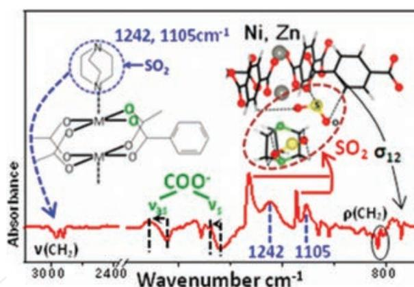
**Figure 10.** Snapshot of initial adsorption configuration models of SO<sub>2</sub> in Zn(bdc)(ted)<sub>0.5</sub> and IR absorption spectra after loading SO<sub>2</sub> at 256 Torr, recorded immediately after evacuation of gas phase (within 16 s). Reprinted with permission from [25]. Copyright (2013) American Chemical Society.
