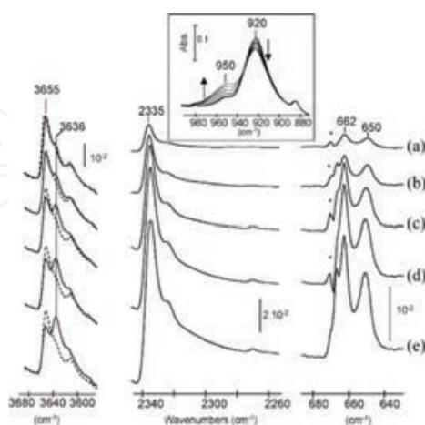
**Figure 3.** CO<sub>2</sub> introduction on MIL-53 (Cr) activated at 473 K. Spectra of activated MIL-53(Cr) deposited on silicon wafer (dotted lines) in three regions and then after introduction of increasing CO<sub>2</sub> equilibrium pressures into the cell (full lines): (a) 1066 Pa, (b) 2400 Pa, (c) 3850 Pa, (d) 5000 Pa, (e) 5850 Pa. Inset: perturbation of the δ(OH) mode upon CO<sub>2</sub> adsorption. Reproduced from [6] with permission of The Royal Society of Chemistry.
