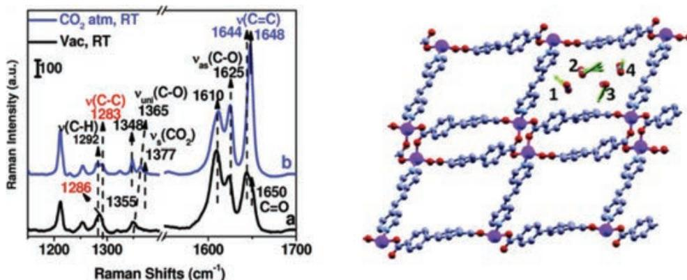
**Figure 5.** (Left) Raman spectra of activated Zn<sub>2</sub>(bpdc)<sub>2</sub>(bpee) in a vacuum and after introduction of 1 atm of CO<sub>2</sub> at room temperature; (right) adsorption sites of CO<sub>2</sub> in complete occupation in Zn<sub>2</sub>(bpdc)<sub>2</sub>(bpee) determined by vdW-DFT, where each pore within a unit cell is occupied by four CO<sub>2</sub> molecules. Reprinted with permission from [12]. Copyright (2011) American Chemical Society.
