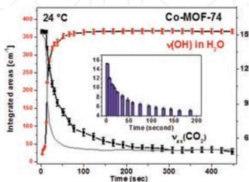
**Figure 12.** Evolution of integrated areas of the IR bands of water  $\nu(\text{OH})$  (red) and CO<sub>2</sub>  $\nu_{\text{as}}(\text{CO}_2)$  (black) in Co-MOF-74 at 24°C. The inset purple bar curve shows the  $\nu_{\text{as}}(\text{CO}_2)$  band evolution corrected by removing the water transport time (taken from the gray curve) and hence provides the intensity evolution solely controlled by exchange kinetics. Reprinted with permission from [31]. Copyright (2015) American Chemical Society.
