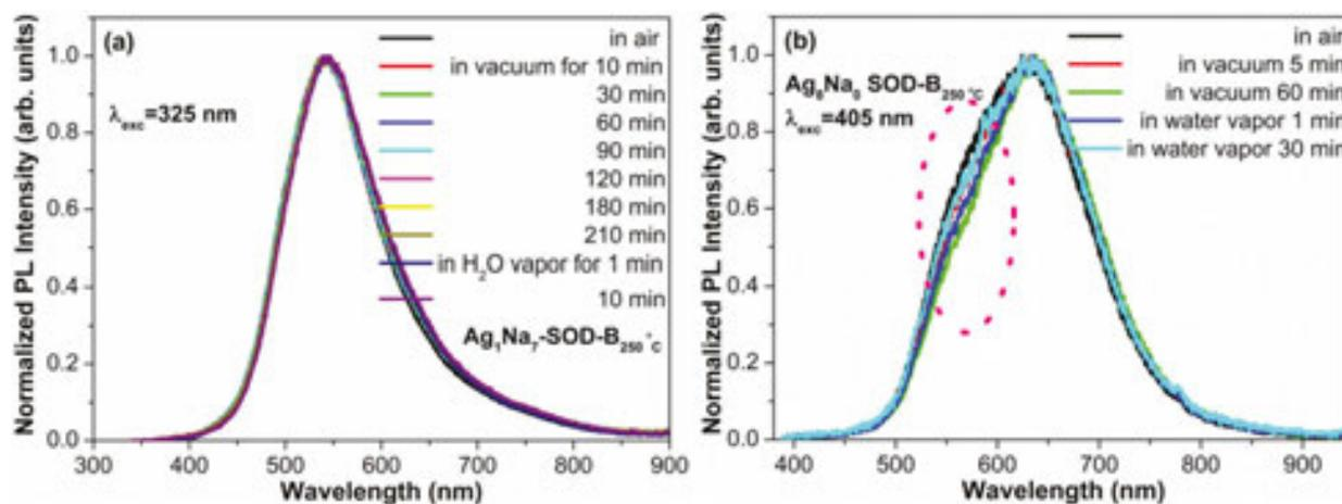
**Figure 10.** PL spectra recorded in different environmental conditions for Ag<sub>1</sub>Na<sub>7</sub>-SOD-B<sub>250°C</sub> (a) and Ag<sub>8</sub>Na<sub>0</sub>-SOD-B<sub>250°C</sub> (b) [38] (reproduced from Royal Society of Chemistry).
