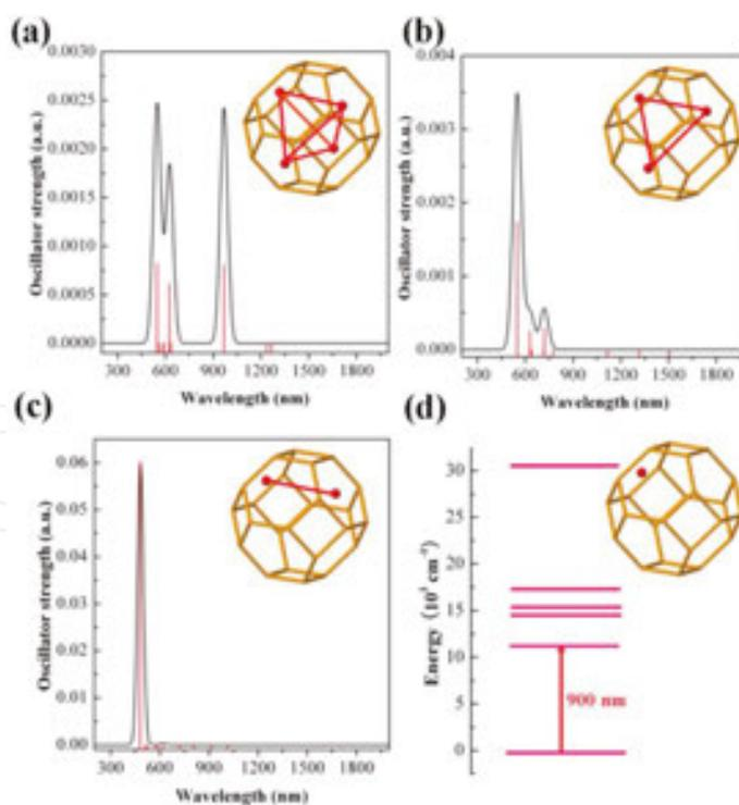
**Figure 5.** Theoretical absorption spectra for  $\text{Bi}_4^{4+}$  (a),  $\text{Bi}_3^{3+}$  (b), and  $\text{Bi}_2^{2+}$  (c). The energy-level diagram of  $\text{Bi}^+$  (d) was drawn according to the experimental absorption spectrum of  $\text{AlCl}_3\text{-NaCl}$  molten salt containing  $\text{Bi}^+$  [21] (reproduced from American Chemical Society).
