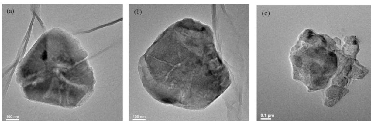
**Figure 1.** TEM morphology of pure zeolite Y (a),  $\text{Nd}^{3+}$  singly exchanged zeolite Y (b), and  $\text{Nd}^{3+}$ ,  $\text{Ag}^+$  ion-exchanged zeolite Y (c) individual particles treated at  $900^\circ\text{C}$  [17] (reproduced from American Institute of Physics).
