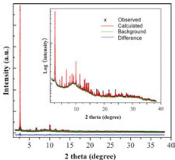
**Figure 4.** Rietveld fit to the high-resolution synchrotron XRD pattern of dehydrated Bi-embedded zeolite Y. Plots show the observed and calculated powder patterns. A difference curve is shown at the bottom of the diagram. Inset: a logarithmic-scale version of the graph [21] (reproduced from American Chemical Society).
