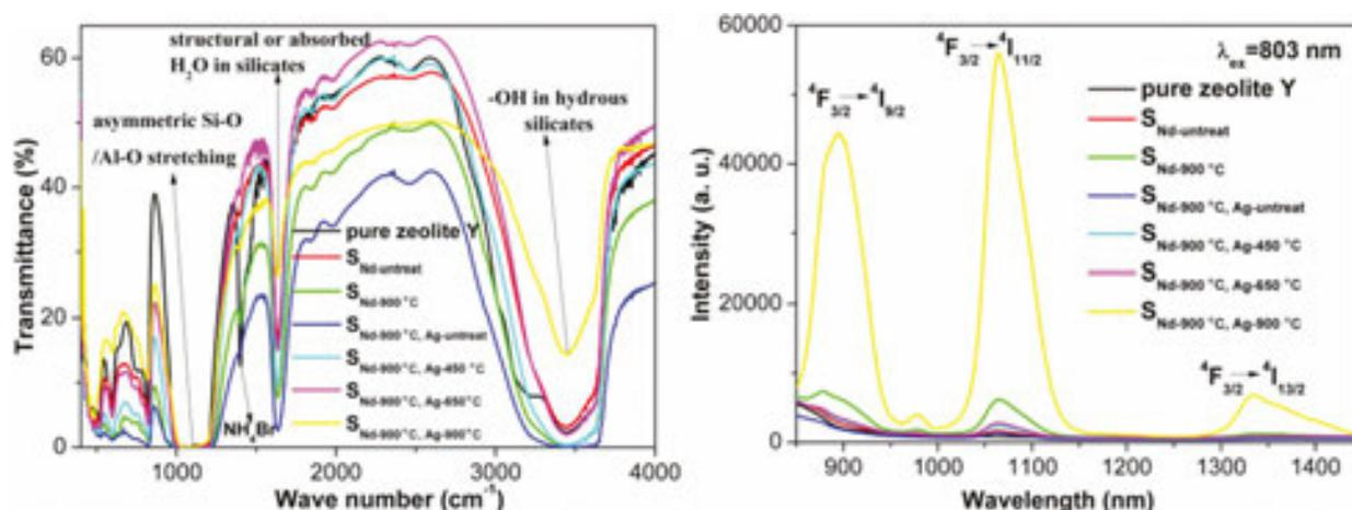
**Figure 2.** Left, FTIR spectra for the pure zeolite Y, Nd<sup>3+</sup> ion-exchanged zeolite Y, and Nd<sup>3+</sup>, Ag<sup>+</sup> ion-exchanged zeolite Y under different thermal treatment conditions; right, NIR emission spectra of the Nd<sup>3+</sup> (and Ag<sup>+</sup>) ion-exchanged zeolite Y samples under different thermal treatment conditions [17] (reproduced from American Institute of Physics).
