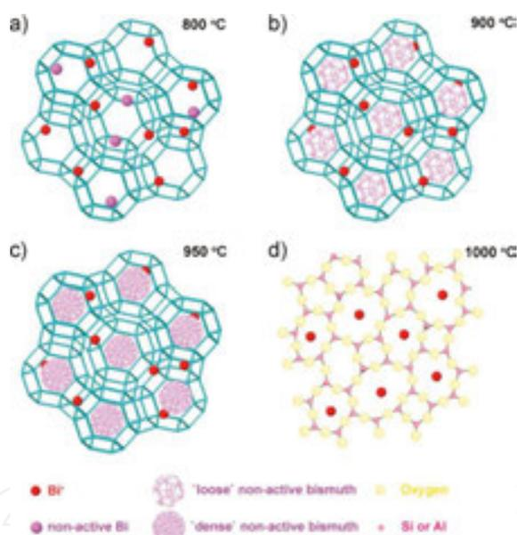
**Figure 3.** (a–c) Schematic illustration of the structure transformation of the zeolites annealed at different temperatures. (d) 2D representation of the structure of an aluminosilicate network. Note that “loose” and “dense” just represent small and large possibilities of sealing the pores of the zeolites with Bismuth agglomerates [15] (reproduced from John Wiley and Sons).
