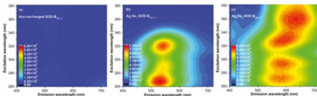
**Figure 9.** Excitation-emission 3D contours of non-exchanged SOD-B<sub>250°C</sub> (a), Ag<sub>1</sub>Na<sub>7</sub>-SOD-B<sub>250°C</sub> (b), and Ag<sub>8</sub>Na<sub>0</sub>-SOD-B<sub>250°C</sub> (c) [36] (reproduced from Royal Society of Chemistry).
