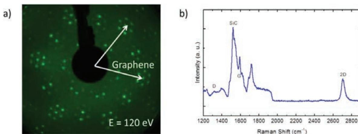
**Figure 1.** (a) Typical LEED image of graphene on SiC(0 0 0 1) and (b) typical micro-Raman spectra of the graphene monolayer. Contributions at the G and 2D bands are observed, together with a very low signal at the defect band D.
