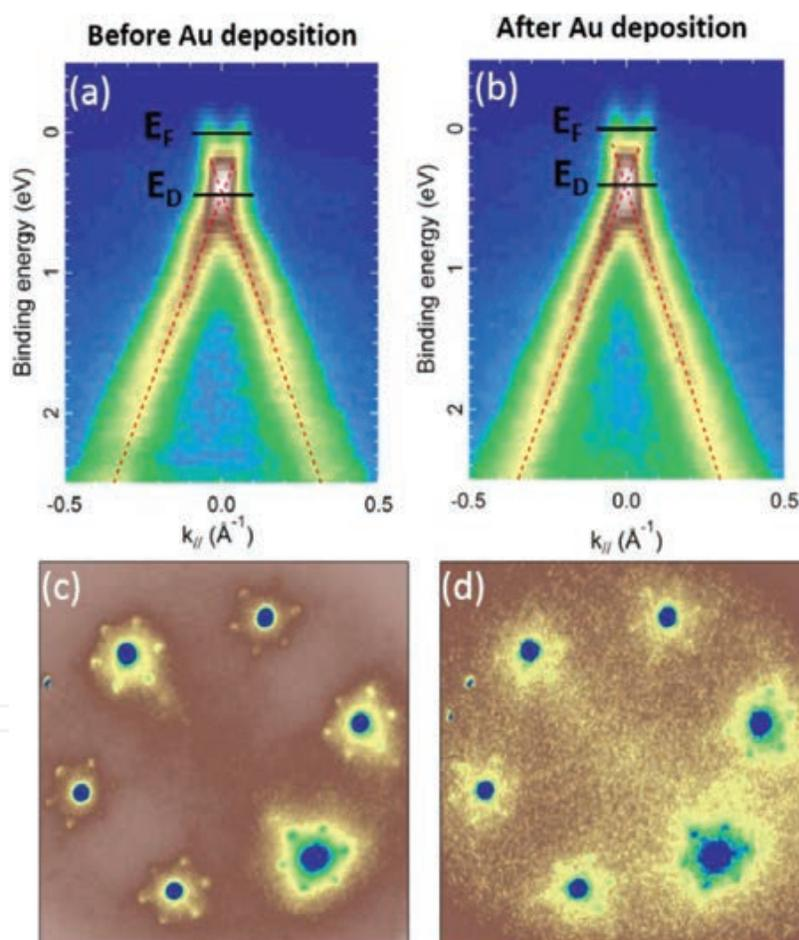
**Figure 4.** Top: band dispersions as a function of  $k_{||}$  around the K point of the first Brillouin zone, obtained by  $\mu$ ARPES at  $h\nu = 40$  eV, performed before (a) and after (b) Au deposition. The Fermi level and the Dirac point are superimposed on the images. Bottom: 2D maps as a function of  $k_x$  and  $k_y$ , recorded for a binding energy of 0.15 eV, that is, close to the Fermi level, before (c) and after (d) gold deposition.
