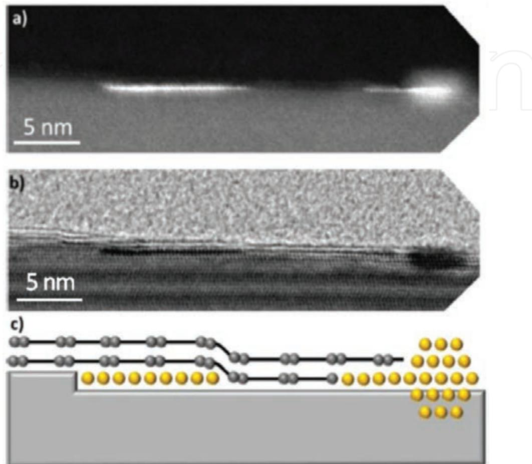
**Figure 6.** Cross-sectional STEM images recorded in the HAADF (top) and bright field (middle) mode, respectively. The substrate, the Au, and graphene layers can clearly be observed. A scheme of the area is also represented (bottom). The substrate is represented by a gray square shape. The Au and carbon atoms are represented by yellow and gray spheres.
