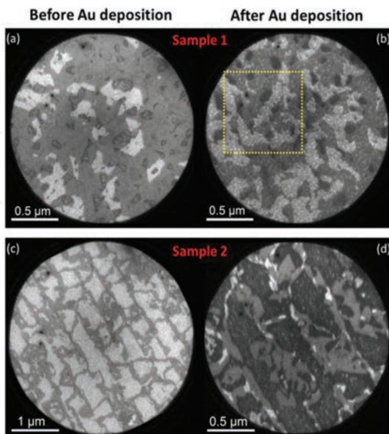
**Figure 2.** LEEM image of a graphene/SiC(0 0 0 1) surface, before (left) and after (right) Au deposition, with an electron beam energy of 3.90 eV. The images for the sample 1 (2) are presented at the top (bottom) of the image.
