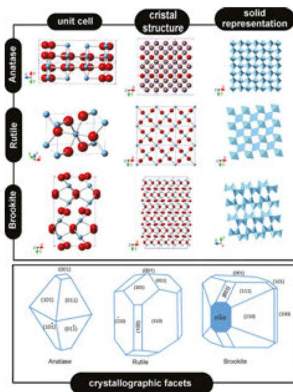
Figure 1. Crystallographic structures of different  $\text{TiO}_2$  crystals: anatase, rutile and brookite.
