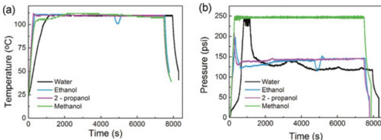
**Figure 7.** Profile of (a) temperature and (b) pressure obtained during TiO<sub>2</sub> nanostructured synthesis with different solvents, water, ethanol, 2 – propanol and methanol, when subject to microwave radiation of 100 W for 120 minutes and a pressure limit of 250 Psi.
