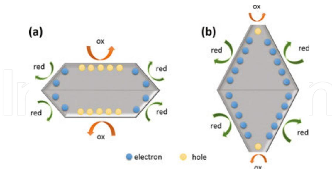
**Figure 3.** Schematic images of spatial separation of redox sites on titanium dioxide structures with a specific exposed crystal facets: (a) larger surface area of oxidation sites (holes) and small surface area of reduction sites (electrons), and (b) smaller surface area of oxidation sites and larger surface area of reduction sites.
