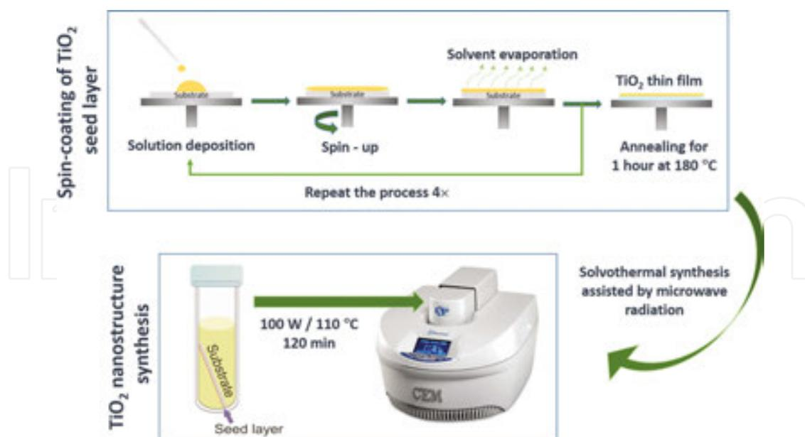
**Figure 5.** Scheme of the TiO<sub>2</sub> seed layer production using the spin-coating method, followed by TiO<sub>2</sub> nanostructured synthesis by solvothermal method assisted by microwave radiation.
