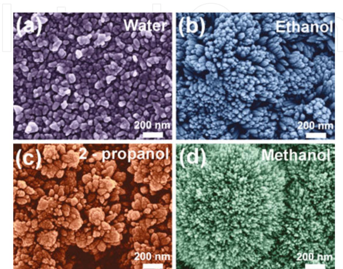
**Figure 8.** SEM images of TiO<sub>2</sub> nanostructures synthesized by solvothermal method, assisted by microwave radiation, using a microwave power of 100 W for 120 minutes and a temperature of 100°C for the solvents tested: (a) water, (b) ethanol, (c) 2 – propanol and (d) methanol. The insets show the cross-section of the produced TiO<sub>2</sub> nanostructures.
