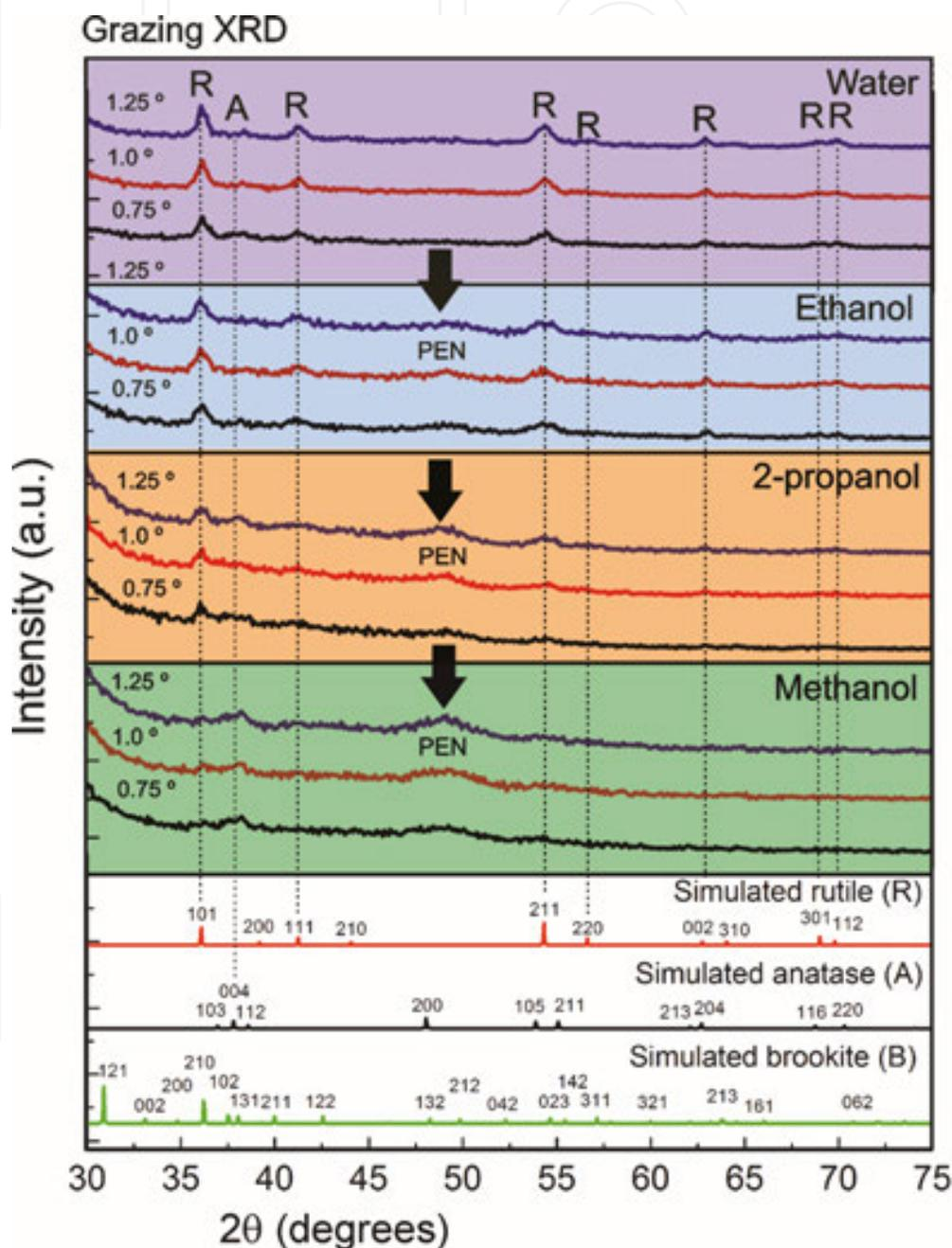
**Figure 9.** Grazing incident XRD diffractograms of TiO<sub>2</sub> nanostructured arrays produced with different solvents: water, ethanol, 2 – propanol and methanol. The grazing incident angles tested were 0.75, 1.0 and 1.25 °. The simulated rutile, anatase and brookite diffractograms are presented for comparison.
