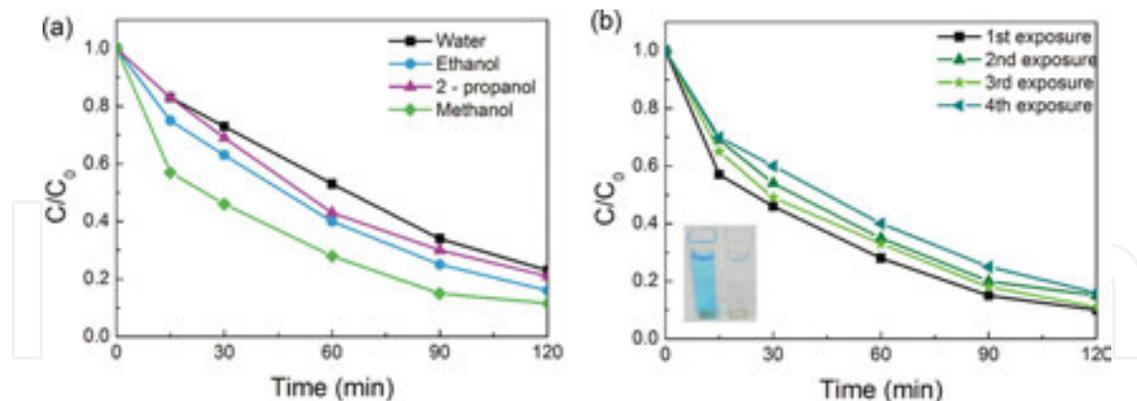
**Figure 12.** (a) MB concentration versus exposure time for the different photocatalysts produced with each solvent tested; (b) MB degradation ratio ( $C/C_0$ ) vs. UV exposure time for the TiO<sub>2</sub> synthesized with methanol, after several UV exposure experiments. On the inset is possible to observe the colour difference in MB before and after the degradation experiment.
