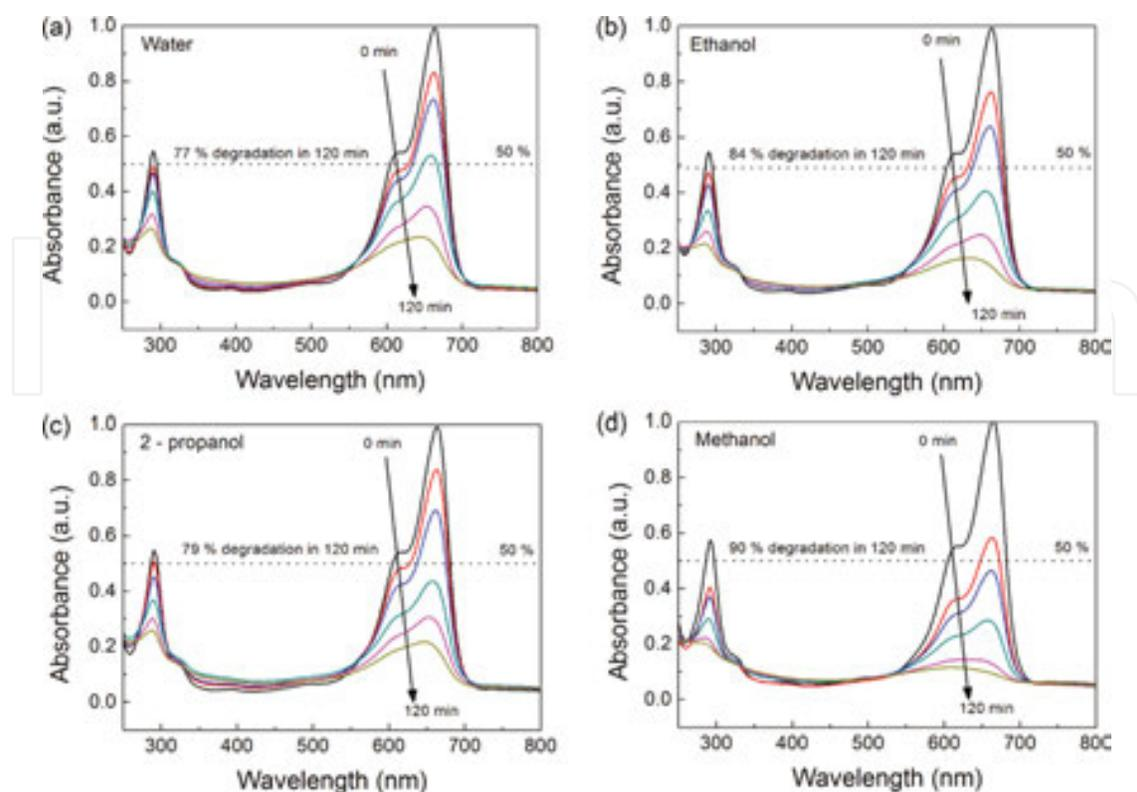
**Figure 11.** Normalized absorbance spectra of MB degradation under UV radiation as a function of exposure time in the presence of each TiO<sub>2</sub> nanostructured arrays synthesized with (a) water, (b) ethanol, (c) 2 - propanol and (d) methanol at room temperature and under an UV radiation of 160 nm, for 120 minutes.
