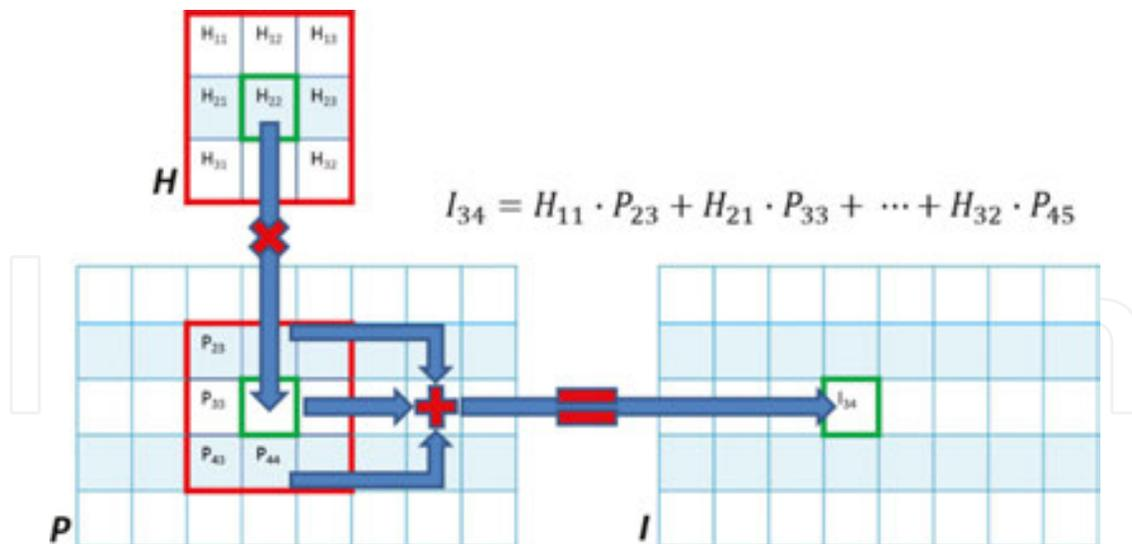
**Figure 9.** Mode of operation of a linear filter [24].
