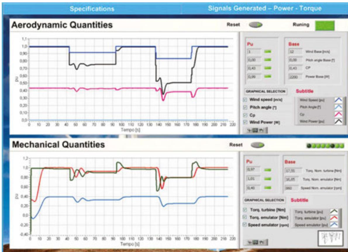
**Figure 11.** Operating dynamics for wind turbine emulation system.
