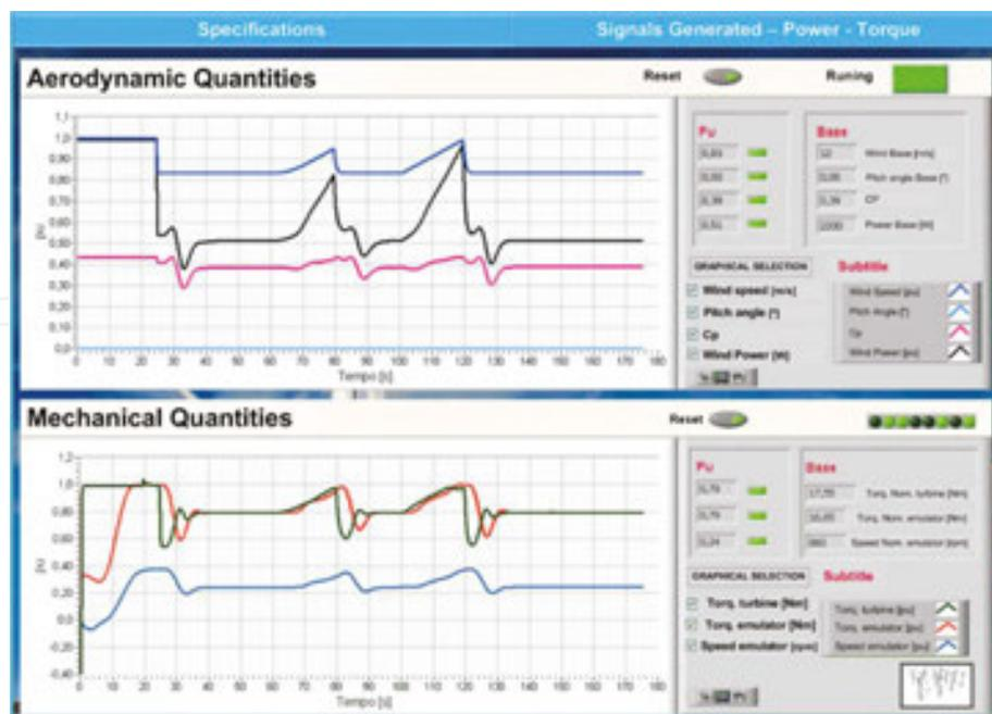
Figure 14. System emulator for the scenario with wind speed ramps.
