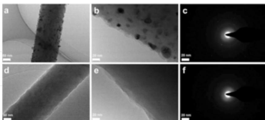
**Figure 9.** (a and b) HRTEM images of SnO<sub>x</sub>/CNFs and (c) corresponding selected area electron diffraction (SAED) pattern; (d and e) HRTEM images of SnO<sub>x</sub>-20%Cu/CNFs and (f) corresponding SAED pattern after 1000-cycle performance test at a current density of 2 A g<sup>-1</sup> [86].
