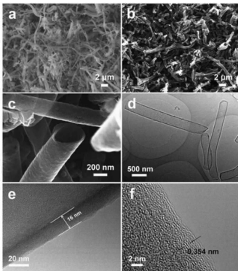
Figure 5. (a) SEM image of  $\text{SiO}_2$  NFs, (b and c) SEM images of N-CTs, and (d–f) HR-TEM images of N-CTs [65].
