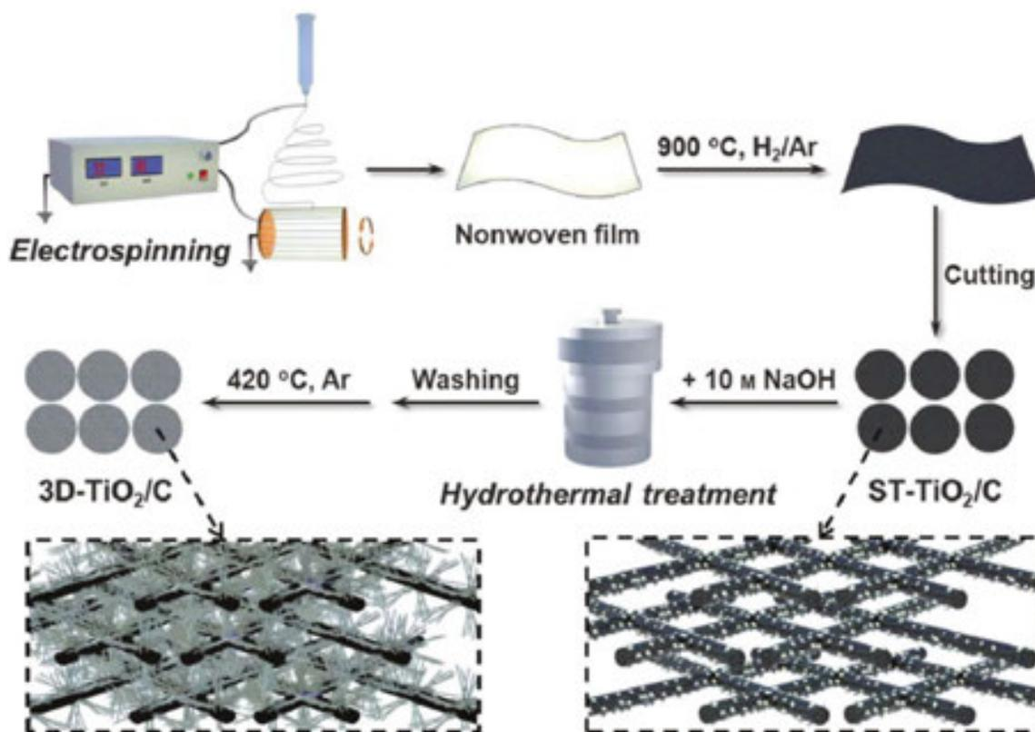
**Figure 11.** Schematic representation of the preparation for the 3D porous  $\text{TiO}_2$  nanotube/carbon nanofiber architecture (ST- $\text{TiO}_2/\text{C}$ : electrospun  $\text{TiO}_2/\text{C}$  nanofibers after calcination as a starting raw material; 3D- $\text{TiO}_2/\text{C}$ : 3D porous  $\text{TiO}_2$  nanotube/carbon nanofiber architecture prepared by a hydrothermal method) [106].
