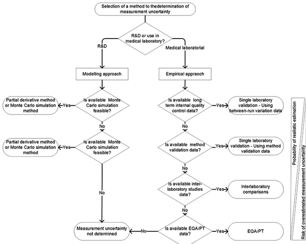
Figure 6. Flow chart to select a model for the determination of measurement uncertainty in a medical laboratory.
