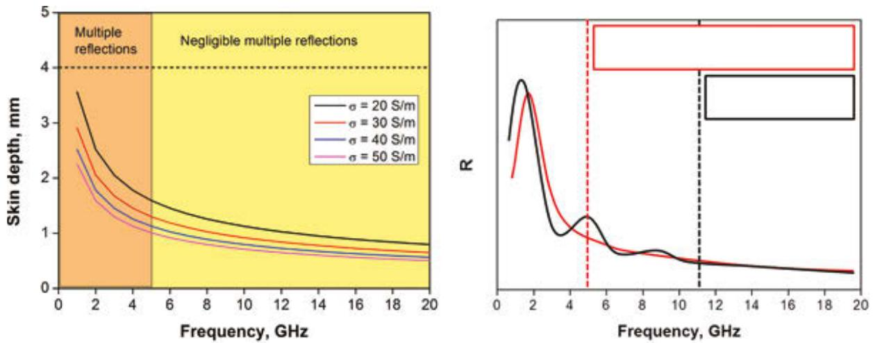
**Figure 4.** (a) Skin depth as a function of frequency for samples with different conductivities. (b) Effect of multiple reflections of two samples with the same thickness and different conductivity. Colored rectangles show the frequency range where multiple reflections are negligible.
