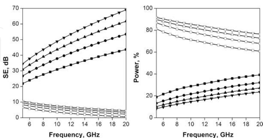
**Figure 6.** Reflection shielding and reflection coefficient ( $R$ ) of specimens with 20 ( $\square$ ), 30 ( $\circ$ ), 40 ( $\Delta$ ) and 50  $\text{S.m}^{-1}$  ( $\nabla$ ). Absorption shielding and transmission coefficient through the first plane of incidence ( $1 - R$ ) of specimens with 20 ( $\blacksquare$ ), 30 ( $\bullet$ ), 40 ( $\blacktriangle$ ) and 50 ( $\blacktriangledown$ )  $\text{S.m}^{-1}$ .
