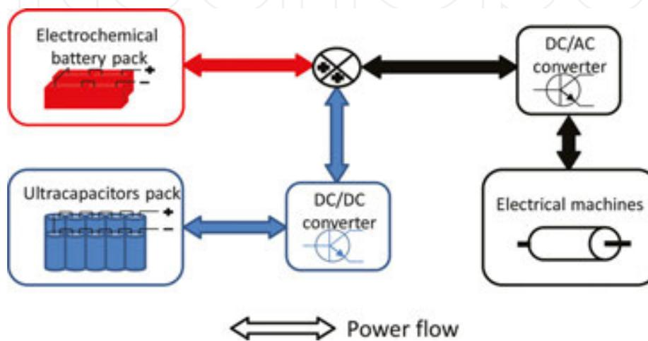
**Figure 1.** Schematic of the BEV power system.
