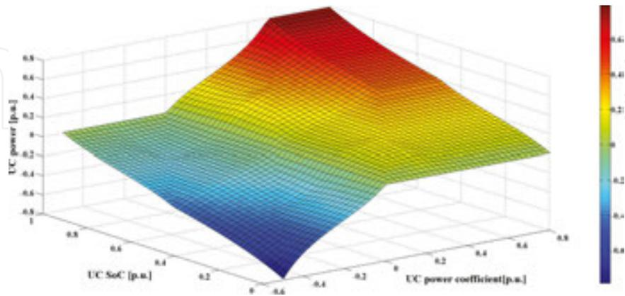
Figure 4. Second level fuzzy logic supervision response surface.
