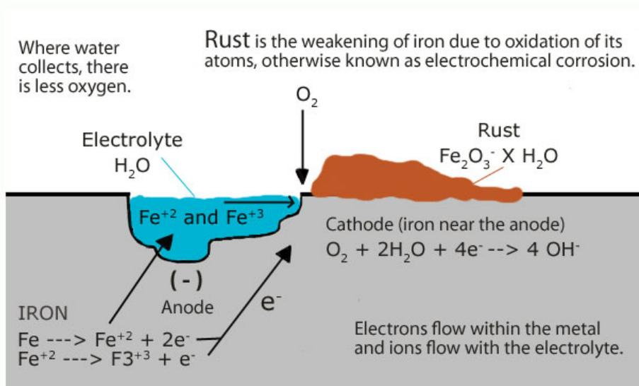
Figure 2. Corrosion Mechanism of Iron to Produce Rust [14].
