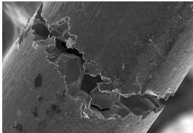
**Figure 5.** Intergranular Corrosion [19].
