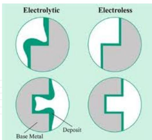
**Figure 9.** Schematic Illustration of Advantage of Electroless Plating [28].
