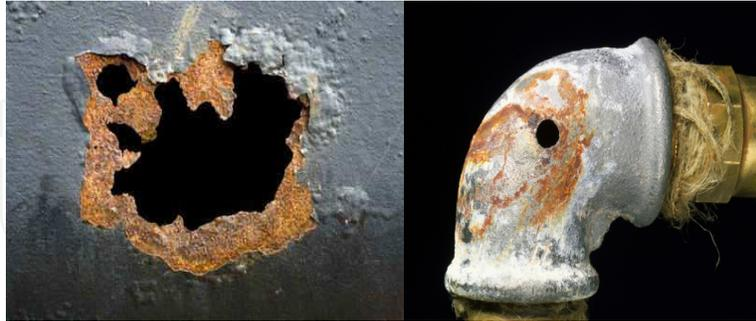
Figure 6. Pitting Corrosion [21].
