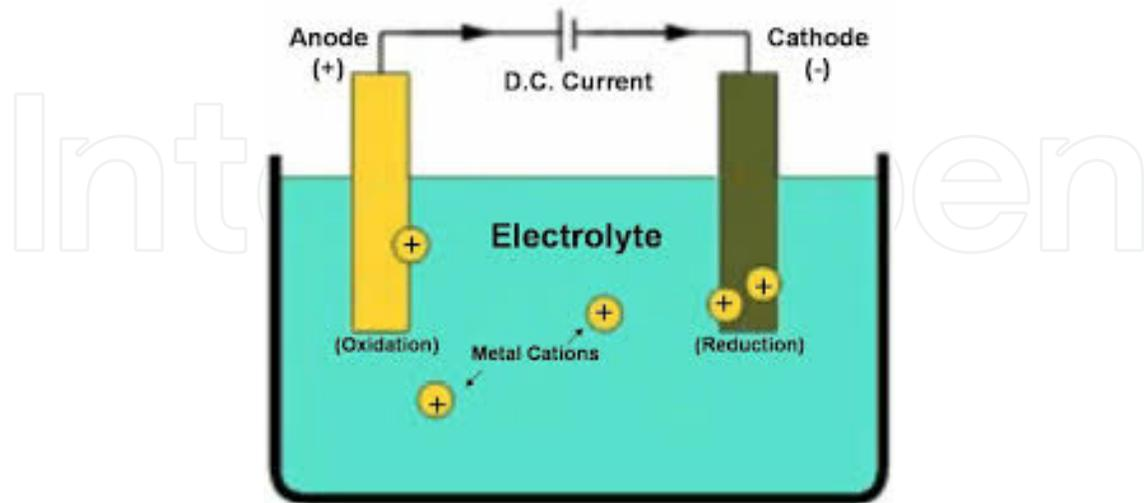
Figure 8. Electrodeposition Setup.
