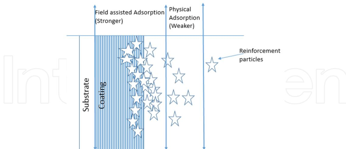
**Figure 2.** Codeposition mechanism into a metal matrix.[50, 51]
