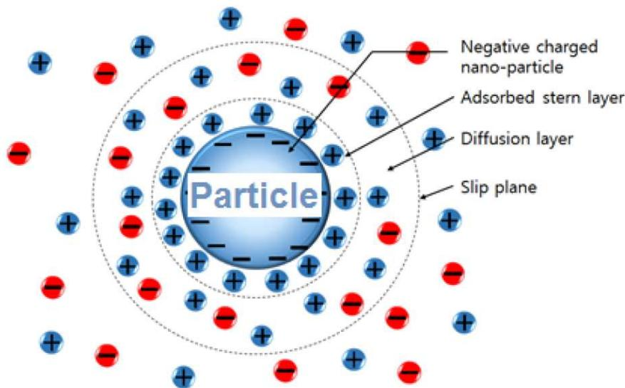
**Figure 3.** Electric double layer around the ceramic particle showing the ionic concentration and generated potential difference as a function of the distance from the charged particle suspended in electrolyte.[51]
