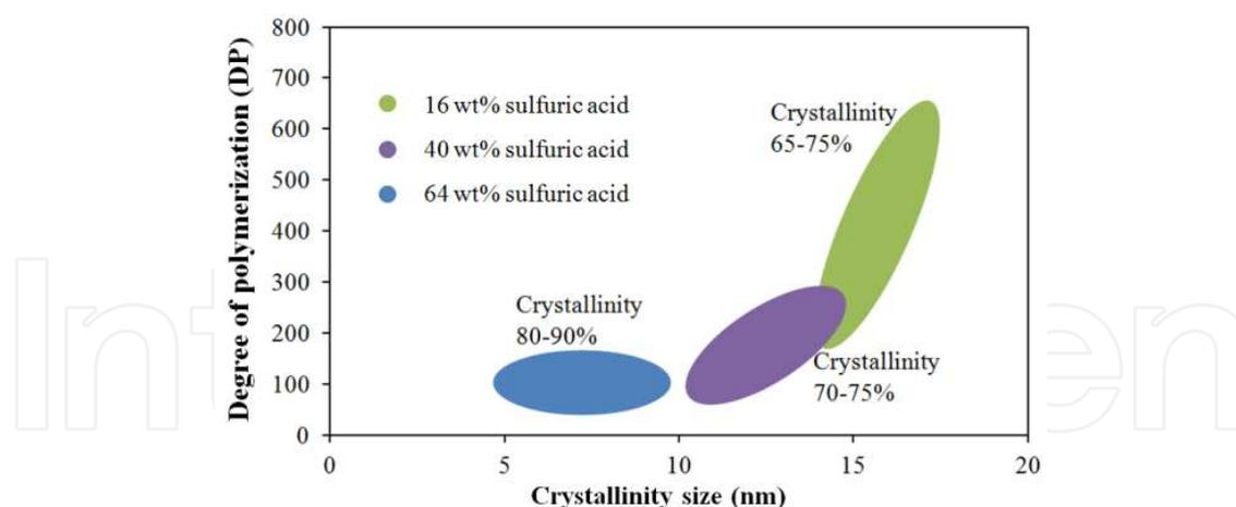
**Figure 6.** Crystallinity size in relation to the DP. During acid hydrolysis, the DP will decrease and the cellulose crystallinity will increase, due to loss of non-crystalline regions and, as a result, smaller crystal size will be obtained.
