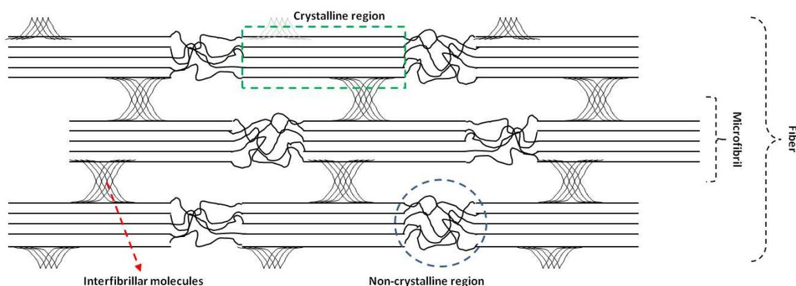
**Figure 3.** Part of a cellulose fiber where the crystalline and non-crystalline regions are shown. Acid hydrolysis removes the non-crystalline regions and only crystalline parts will remain (CNC). Mechanical treatment of the fibers will remain both the non-crystalline and the crystalline regions but some of the interfibrillar bonds will break, creating fibrils in nanometer size in width and micrometer size in length (CNF).
