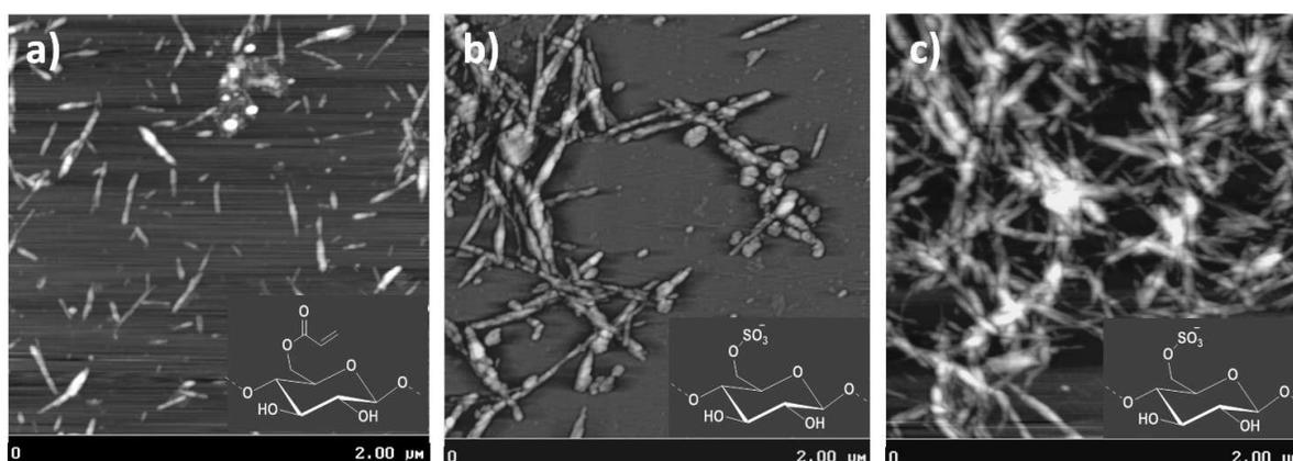
**Figure 7.** AFM picture of CNC from (a) acrylamide sulfate hydrolyzed MCC and a schematic picture of CNC with an acrylate functional group, (b) AFM picture of CNC that has been fully dried, and (c) dried to a high viscous gel. All the crystal dimensions are within nanometer size.
