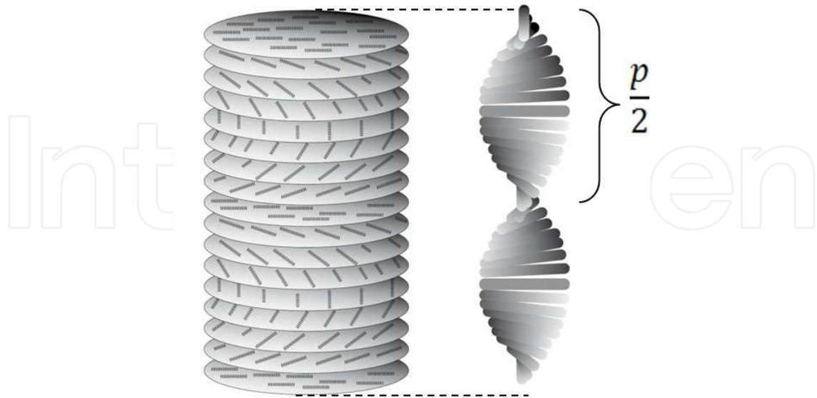
**Figure 4.** At certain concentrations, the nanocrystals self-organize into a chiral nematic ordering where the length of the pitch gap ( $p$ ) in the helical structure can absorb different wavelengths and emit wavelengths with different colors. *Illustration: Jari Sundqvist.*
