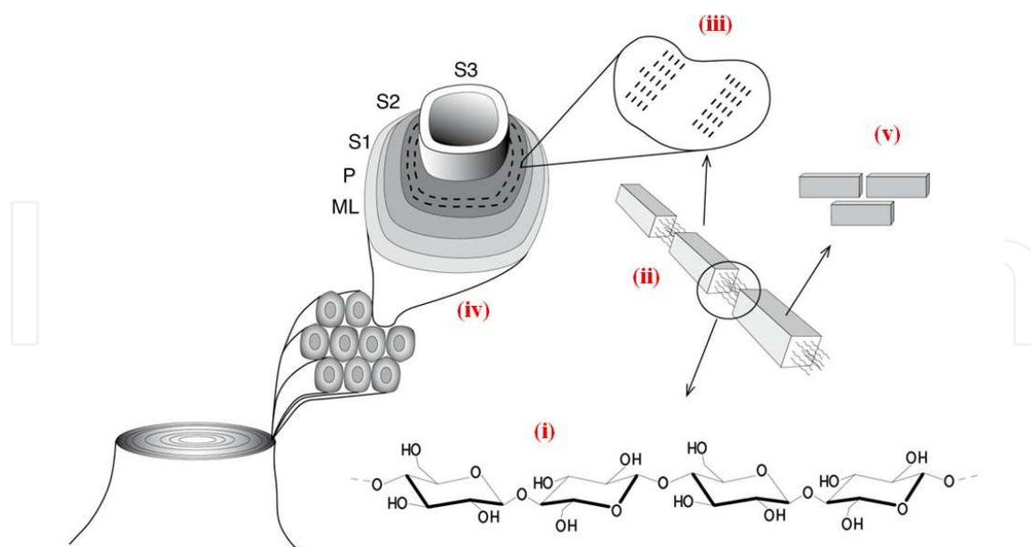
**Figure 2.** The different levels of the cellulose structure: (i) the molecular structure of a cellulose polymer, (ii) the polymers ordered into microfibrils with crystalline and non-crystalline regions, (iii) several microfibrils assembled together to form a macrofibril, and (iv) the different layers in the cell wall. Numbers (ii) and (v) show cellulose microfibrils (CMFs) and cellulose nanocrystals (CNCs), respectively. *Illustration: Jari Sundqvist.*
