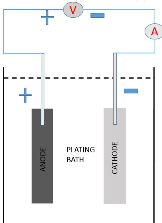
**Figure 1.** A schematic for the electrodeposition process.
