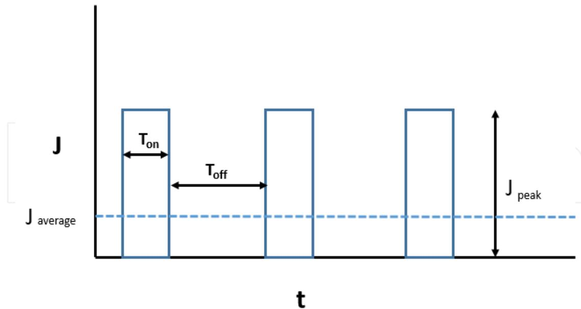
**Figure 3.** Schematic diagram of pulsed current waveform.
