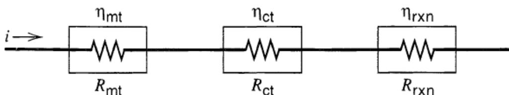
**Figure 2.** Processes in an electrode reaction represented as resistances (From A.J. Bard, and L.R. Faulkner, Chapter 1: Introduction and Overview of Electrode Processes, Page 24, Electrochemical Methods - Fundamentals and Applications, 2<sup>nd</sup> Edition. Reprinted by permission of John Wiley & Sons, Inc. Copyright 2001 © John Wiley & Sons, Inc.
