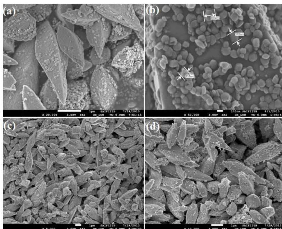
**Figure 2.** Low and high magnification SEM images of self-assembled nanoparticle sheathed  $\text{Fe}_0\text{Gd}_{0.5}(\text{MoO}_4)_{1.5}:\text{Eu}^{3+}$  structures synthesized at (a, b) 24 and (c, d) 48 h.
