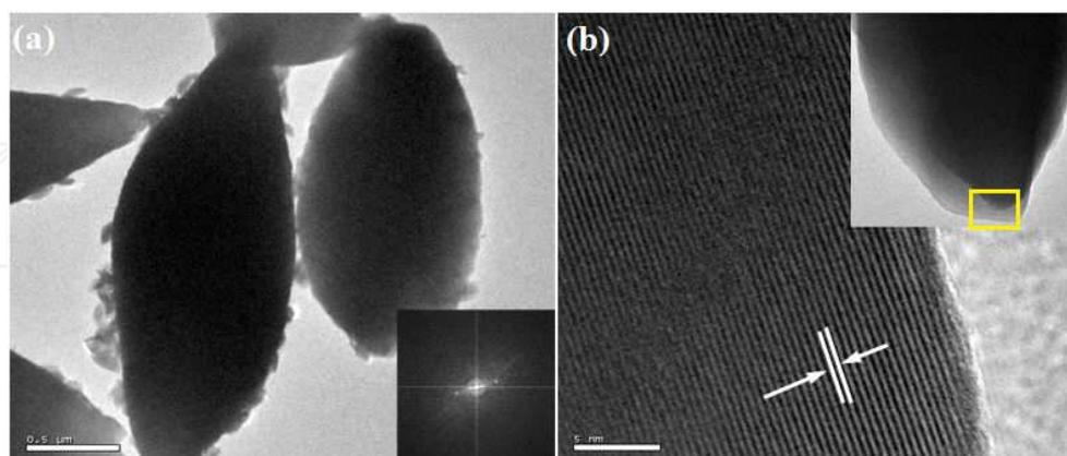
**Figure 3.** (a) TEM image of the  $\text{Fe}_{0.5}\text{Gd}_{0.5}(\text{MoO}_4)_{1.5}:\text{Eu}^{3+}$  sample prepared at 24 h time interval and the corresponding inset shows the FFT pattern, (b) HRTEM image (inset typical HRTEM image taken on the marked part).
