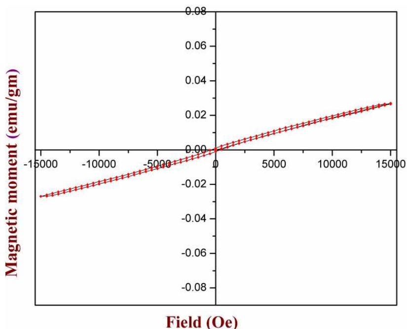
**Figure 8.** Magnetization vs. magnetic field of the as-synthesized bipyramid-like structures of  $\text{Fe}_{0.5}\text{Gd}_{0.5}(\text{MoO}_4)_{1.5}:\text{Eu}^{3+}$  synthesized by hydrothermal treatment at  $200^\circ\text{C}$  for 24 h.
