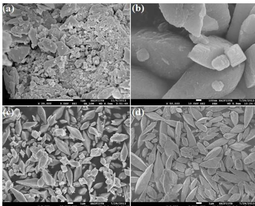
**Figure 1.** Field emission scanning electron microscopic images of  $\text{Fe}_{0.5}\text{Gd}_{0.5}(\text{MoO}_4)_{1.5}:\text{Eu}^{3+}$  synthesized by PVP employed hydrothermal method with different time intervals, i.e., (a) 1 h, (b) 2 h, (c) 6 h, (d) 12 h at 200°C with fixed pH (~7).
