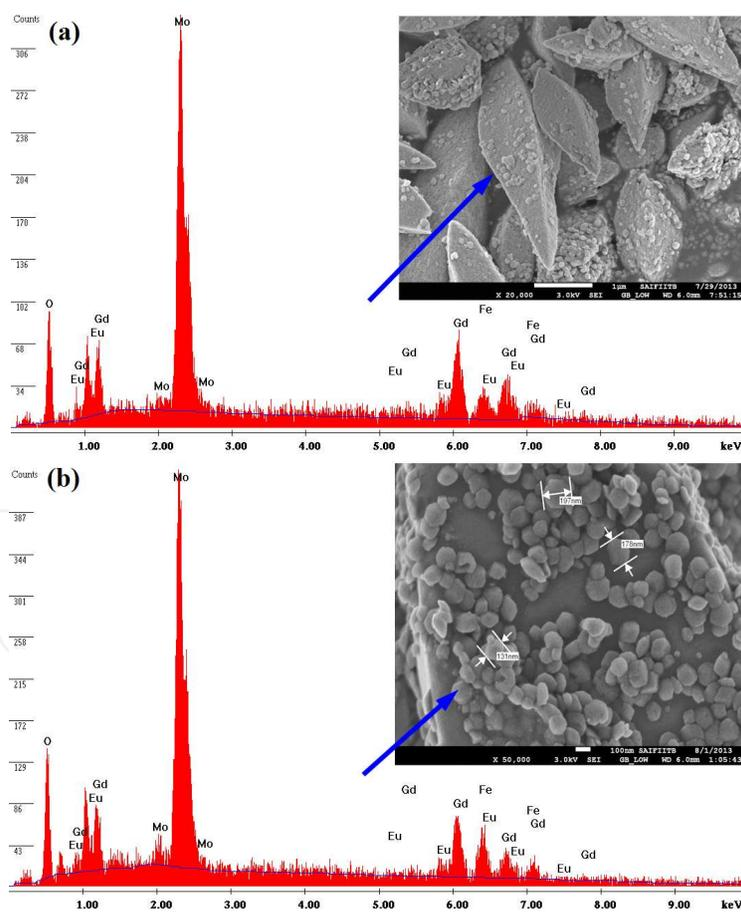
**Figure 6.** (a) EDX spectrum of single bipyramid-like  $\text{Fe}_{0.5}\text{Gd}_{0.5}(\text{MoO}_4)_{1.5}:\text{Eu}^{3+}$  particle, (b) EDX spectrum of single nanoparticle sheathed on a bipyramid-like particle.
