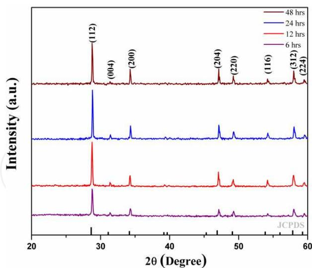
**Figure 5.** Powder X-ray diffraction (XRD) patterns of the  $\text{Fe}_{0.5}\text{Gd}_{0.5}(\text{MoO}_4)_{1.5}:\text{Eu}^{3+}$  samples synthesized at different time intervals using the PVP-mediated hydrothermal method.
