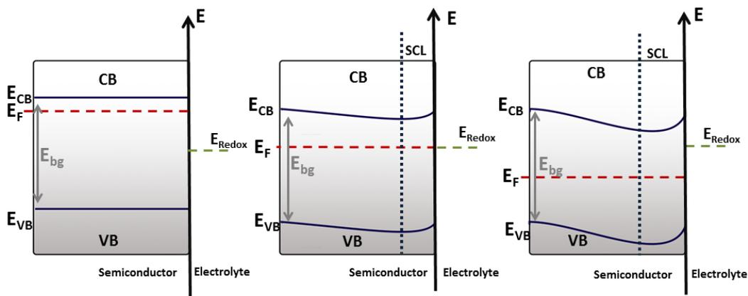
**Figure 4.** Energy diagram of n-type ( $TiO_2$ ) semiconductor in different situations: before semiconductor-electrolyte contact, equilibrium established after semiconductor-electrolyte contact and applying anodic bias.
