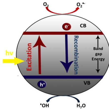
Figure 2. Schematic representation of a photoexcited semiconductor
