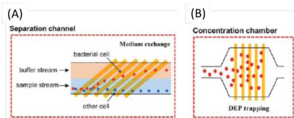
**Figure 5.** Scheme of the microfluidic device presented by Park et al. [59]. In scheme (A), the deviation of bacterial cells from the sample stream is represented, to be incorporated to the buffer stream that brings bacteria to the concentration chamber (B). Adapted from Park et al. [59], with permission of the Royal Society of Chemistry.
