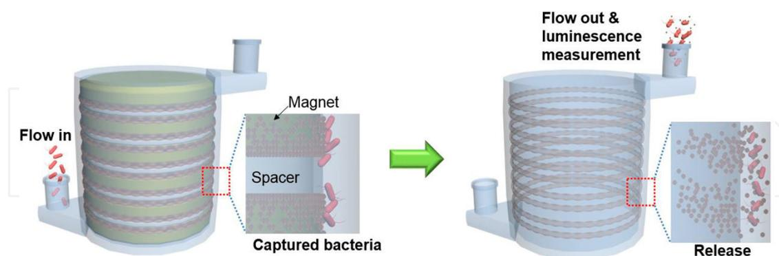
**Figure 1.** Schematic illustrations of 3D immunomagnetic flow assay. The magnet-spacer assembly was placed in the center opening during the capture and rinsing of the magnetic particles and the antibody–*Salmonella* complexes, which were trapped. After removing the magnet assembly from the center opening, the concentrated AbMNC–*Salmonella* solution was collected using a disposable syringe. Reprinted with permission from Lee et al. [36]. Copyright 2014, American Chemical Society.
