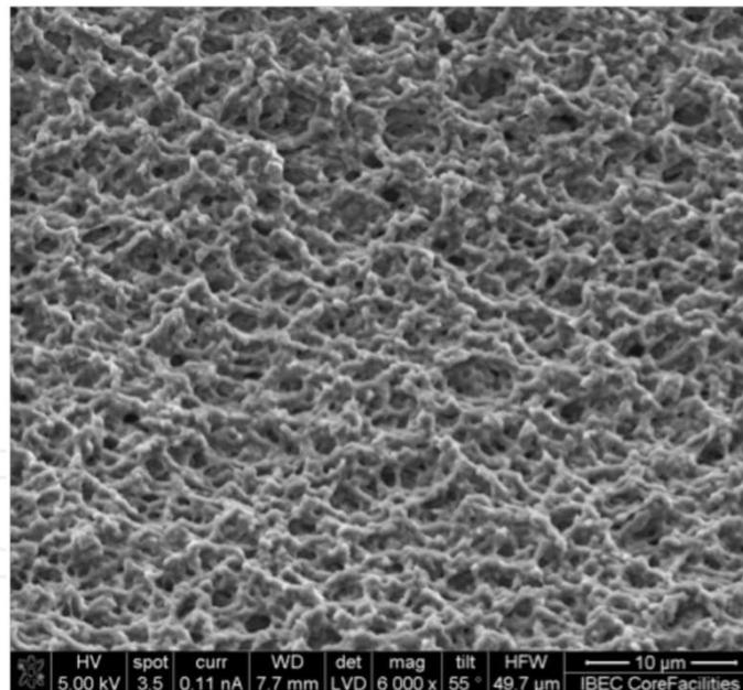
**Figure 4.** Bio-inert polyethylene glycol (PEG)-based hydrogels have been designed as the scaffold substrate for biomimetic matrices supporting muscle migration in three dimensions. The picture shows PEGDA hydrogel (MW 550 KDa) cross-linked by UV light.
