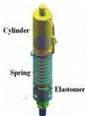
Fig. 15. Damper device for lower limb prosthetics
