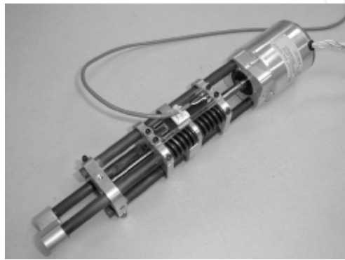
Figure 4. Series elastic actuator with electric motor (reproduced from Robinson, 2000)
