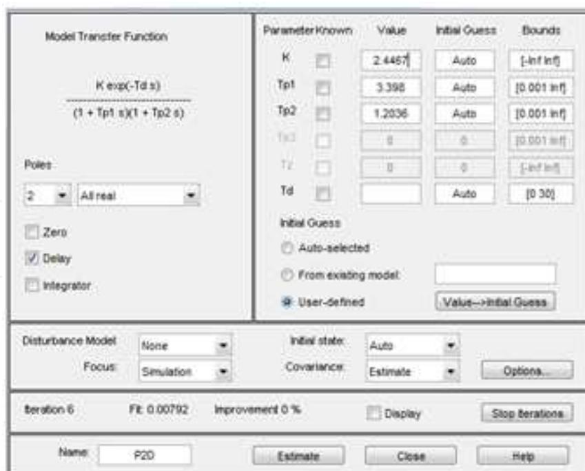
Figure 6. The modeling parameter of the train
