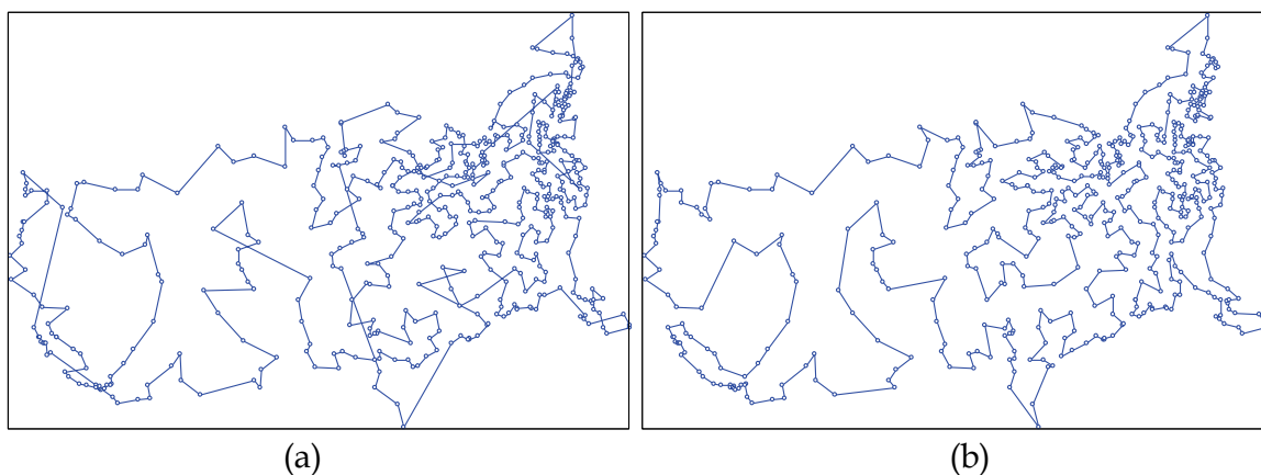
Fig. 6. Solutions found to att532 data. (a) Feasible solution found without local search improvement with 411 epochs and average error of 14.58%. (b) Feasible solution found with local search improvement with 427 epochs and average error of 1.27%.
