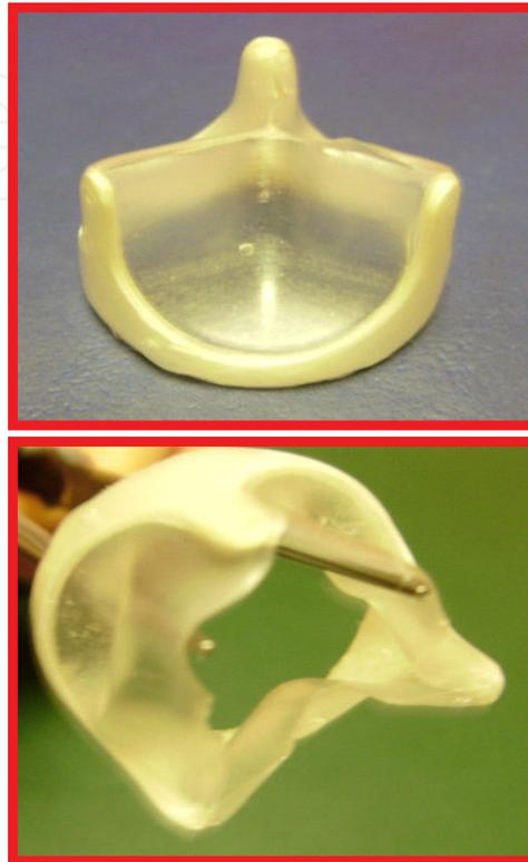
**Figure 8.** Prototype of *Segmented Polyurethane (SPU)* prosthesis.
