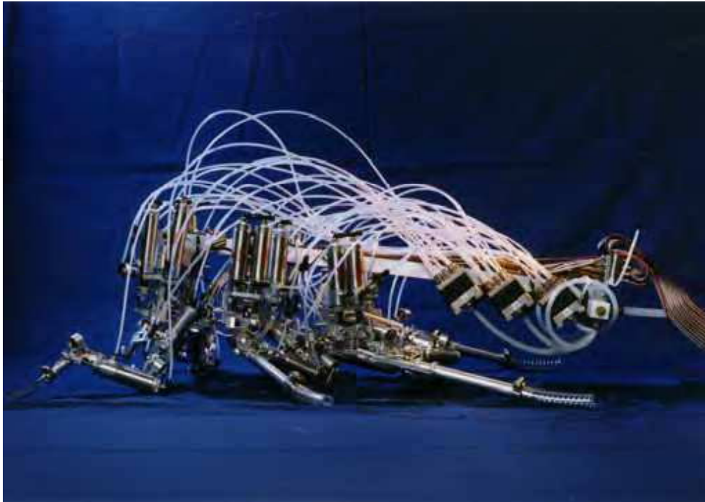
Figure 2. Robot III, a pneumatically powered hexapod modeled structurally and functionally after a cockroach. Robot III was developed at Case Western Reserve University through a long standing collaboration between Roger Quinn's Biorobotics Lab and Roy Ritzmann's neurobiology and behavior lab. Based upon biological data from James Watson, it was designed by Richard Bachmann and Gabriel Nelson with control software by Nelson. (Photo © by and used by permission of R. Quinn. From Quinn et al., 2001, Figure 2, Courtesy of Springer Verlag.)
