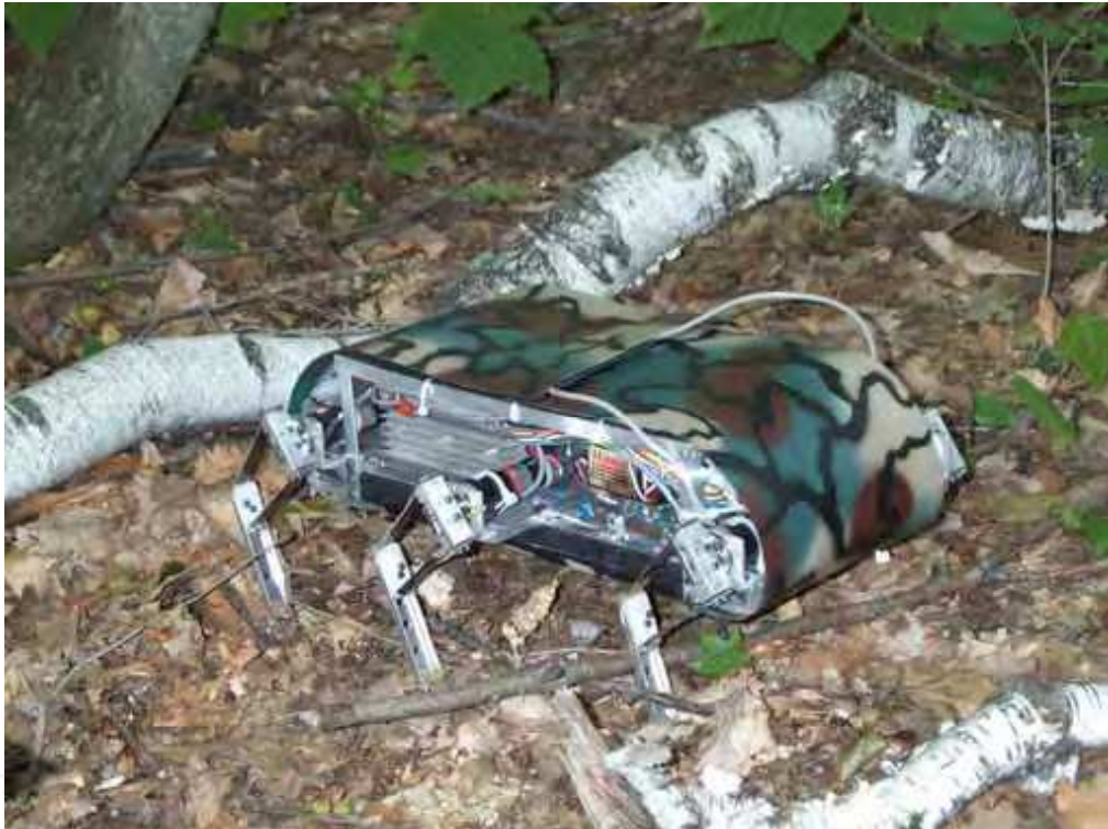
Figure 1. The hexapod robot RHex. Note that although the configuration of the body and the legs does not emulate its model organism, a cockroach, its biomechanics does incorporate the swing inverted pendulum mechanical motion that cockroaches and other insects use. (Photo provided by M. Buehler. Photo © by M. Buehler. Used by permission.)
