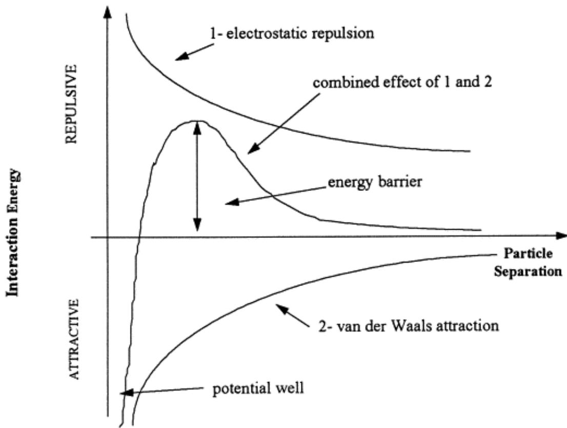
Figure 2. Energy curve of interaction forces [33]
