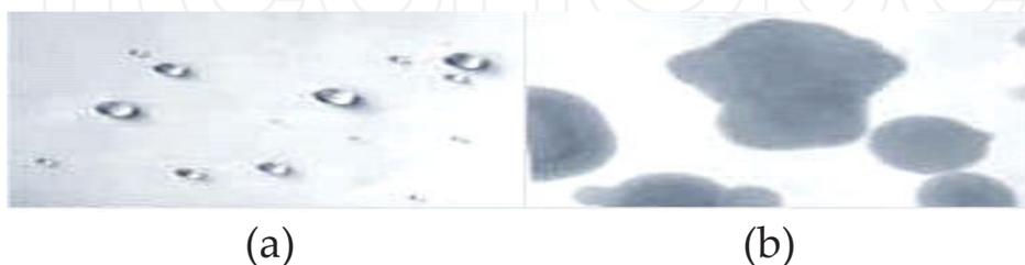
**Figure 4.** a) Hydrophobic membrane, (b) Hydrophilic membrane [14]
