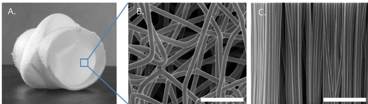
**Figure 4.** (A) Photograph of an electrospun poly( $\epsilon$ -caprolactone) heart valve demonstrating 3D valve architecture, and scanning electron micrographs of its microstructure showing either random (B) or aligned microfibers (C) (scalebar = 100  $\mu\text{m}$ ; images courtesy of M. Simonet and G. Argento).
