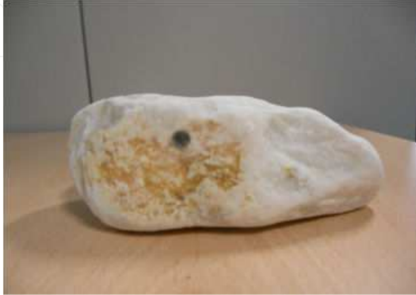
Figure 3. A Smart Pebble. On its surface is possible to notice the hole housing the transponder
