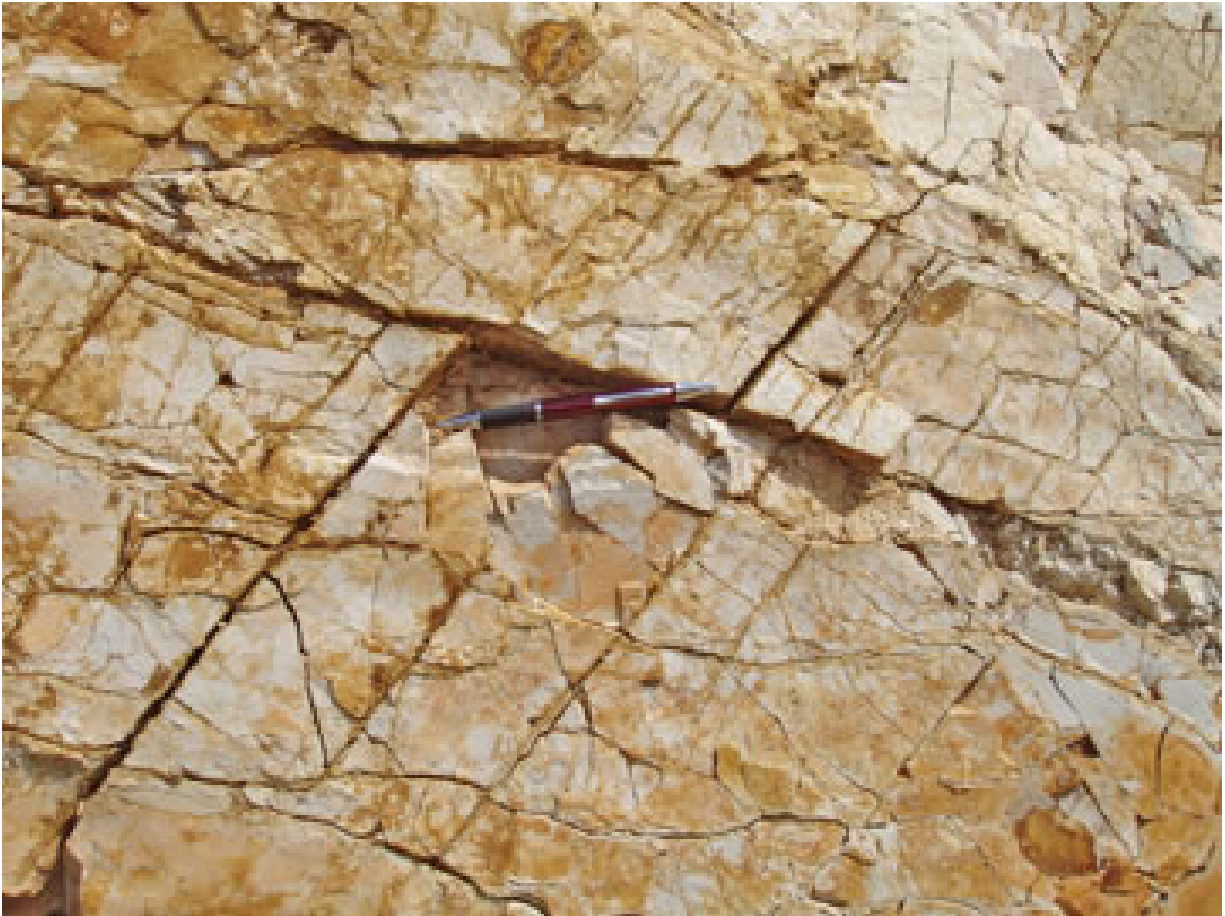
Figure 2. Natural fractures present in a wide range of size and spacing. A pen is used as the scale in this outcrop picture. Depending on the magnitude of induced stresses and others conditions only a portion of these cracks may be reactivated. Effective contact area is determined based on the population of opened fractures (Photo courtesy of Brian Cardott. [25])
