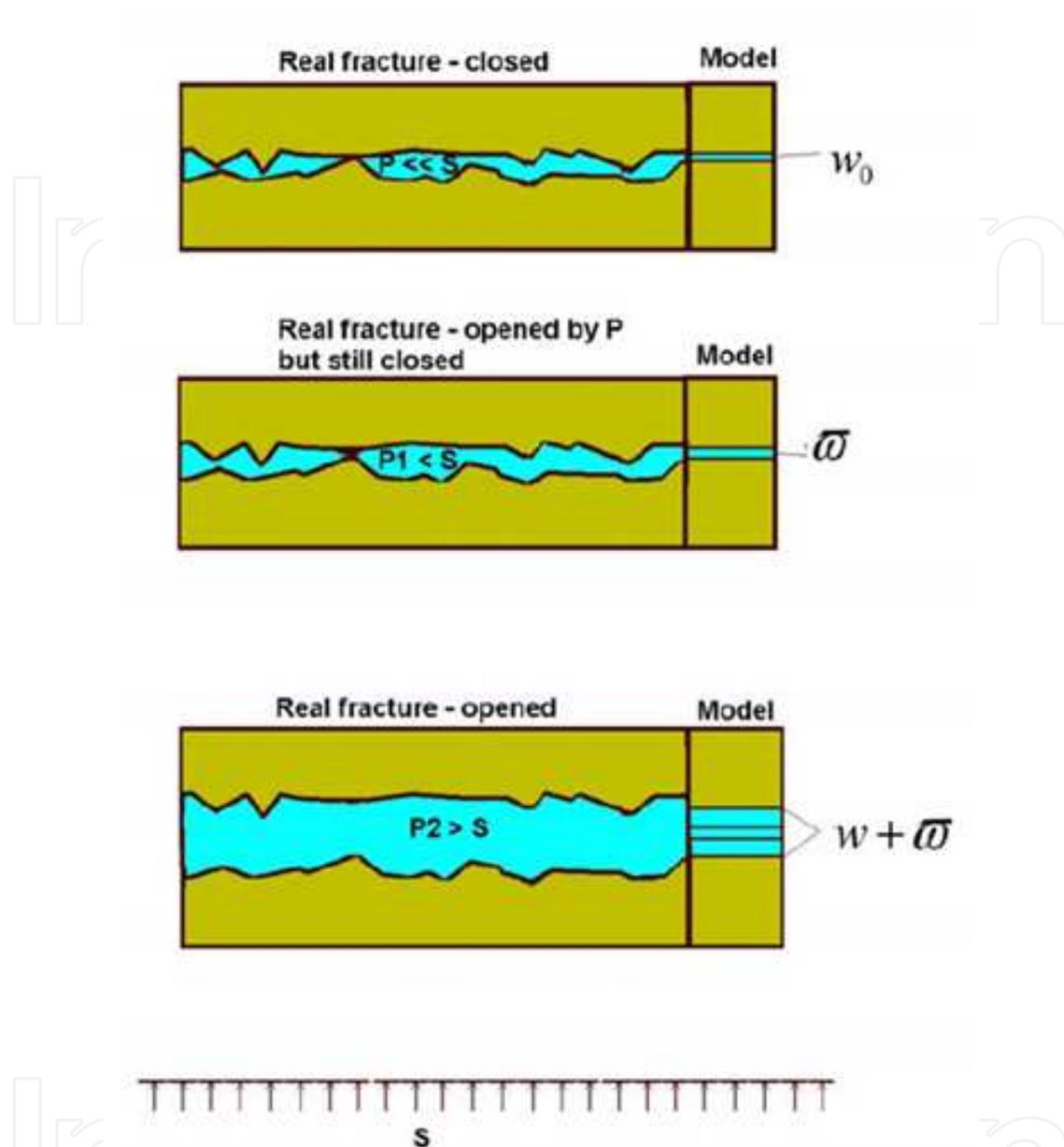
**Figure 1.** Evolution of natural fracture opening [10]
