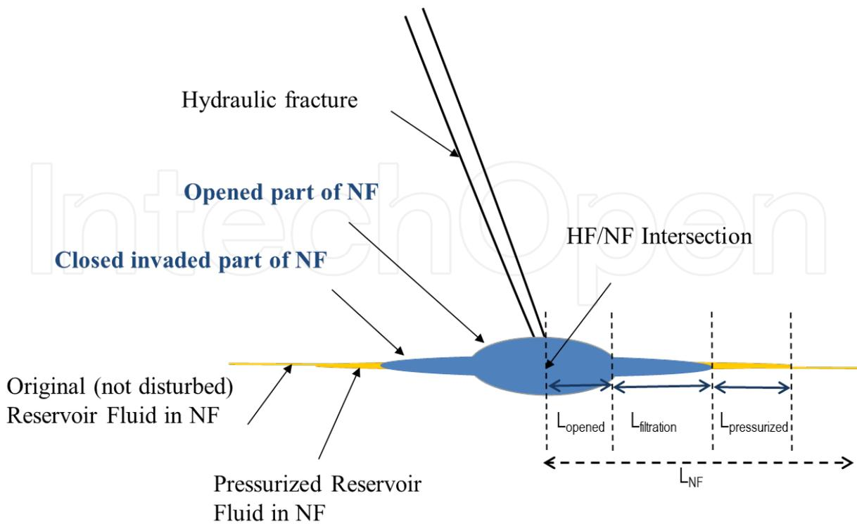
**Figure 4.** Details on different possible zones in intercepted permeable NF
