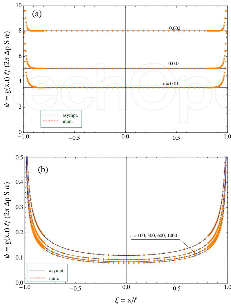
**Figure 2.** Comparison of the numerical solution for the normalized leak-off rate in the auxiliary problem (step pressure increase along the crack) with the small time (a) and large time (b) asymptotes.
