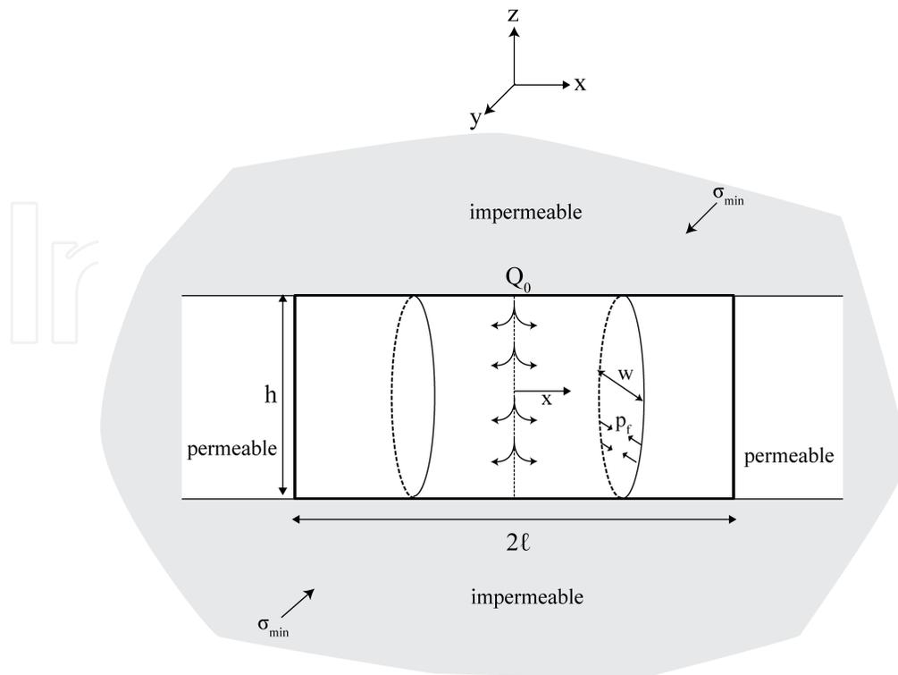
**Figure 1.** A pre-existing PKN fracture with length  $2\ell$  and height  $h$
