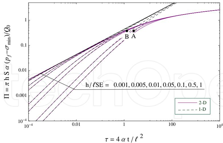
**Figure 3.** Evolution of the fluid net-pressure during a constant-rate injection into a stationary crack within an abnormally-pressurized reservoir  $p_0 \approx \sigma_{min}$  for various values of the crack height-to-length ratio  $h/\ell SE'$ .
