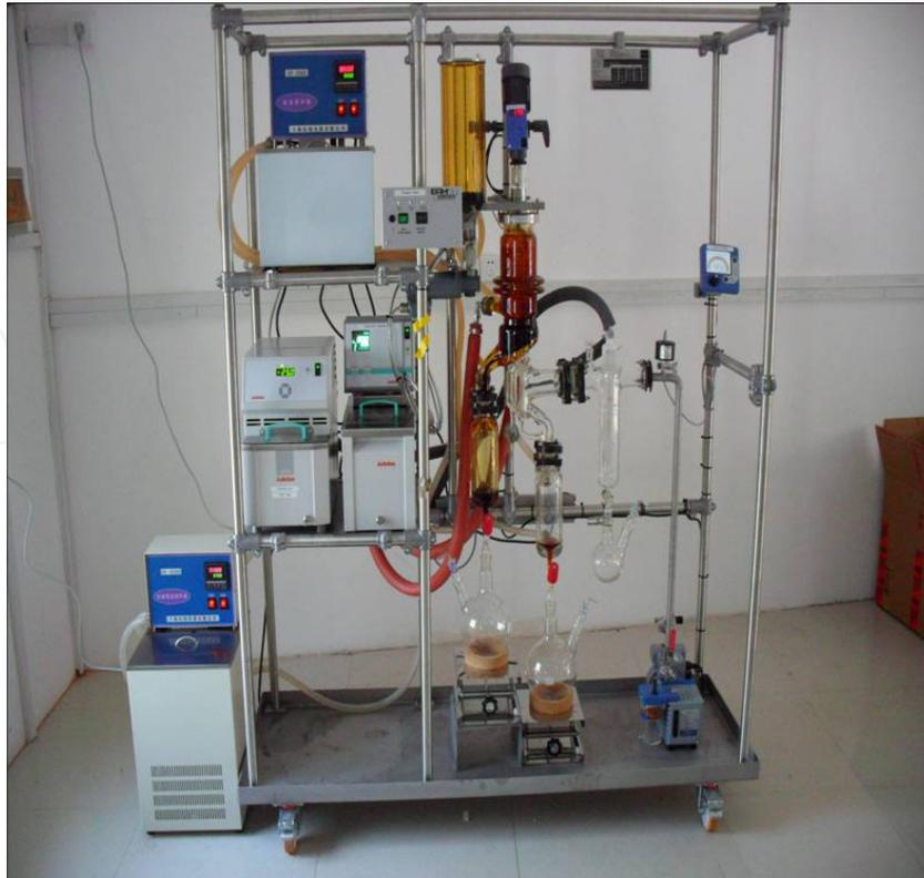
**Figure 2.** KDL-5 molecular distillation apparatus.
