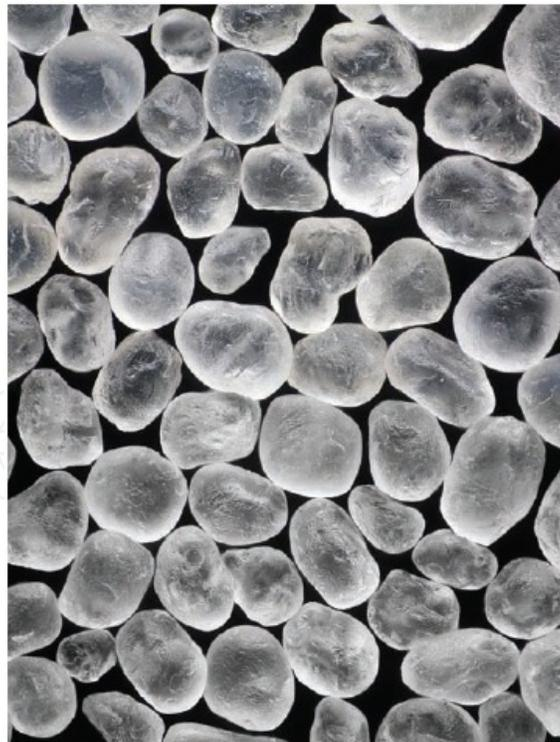
**Figure 2.** Northern White Sand, sphericity ~ 0.73 – Photo courtesy: Santrol.
