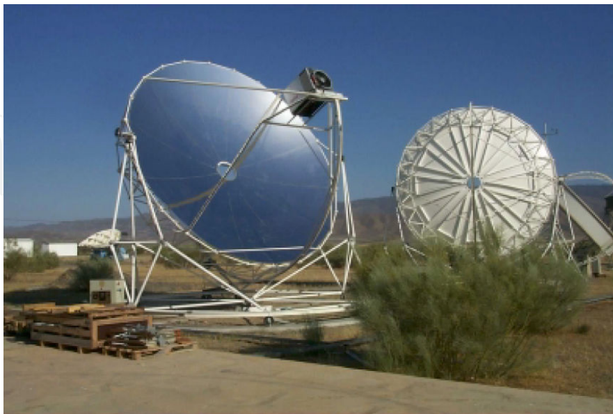
Figure 2. General description of Stirling EuroDish system [12]
