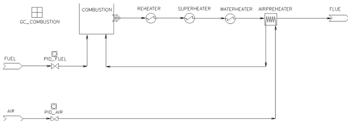
**Figure 5.** Boiler Combustion Model
