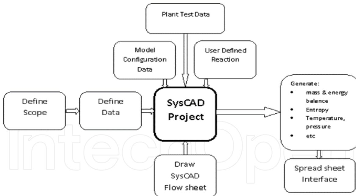
Figure 2. SysCAD Modeling [2]
