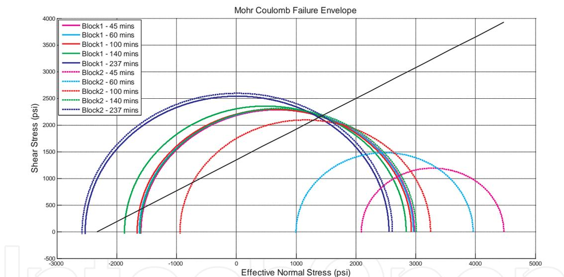
**Figure 7.** Mohr – Coulomb failure envelope for  $C_0=4657\text{psi}$  – Well A
