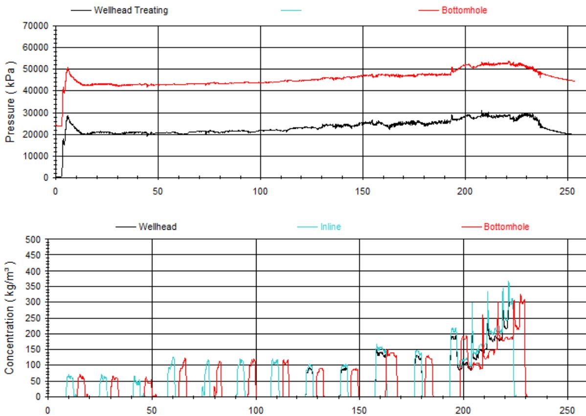
**Figure 1.** BHIP, Wellhead pressure and Proppant concentration - Well A
