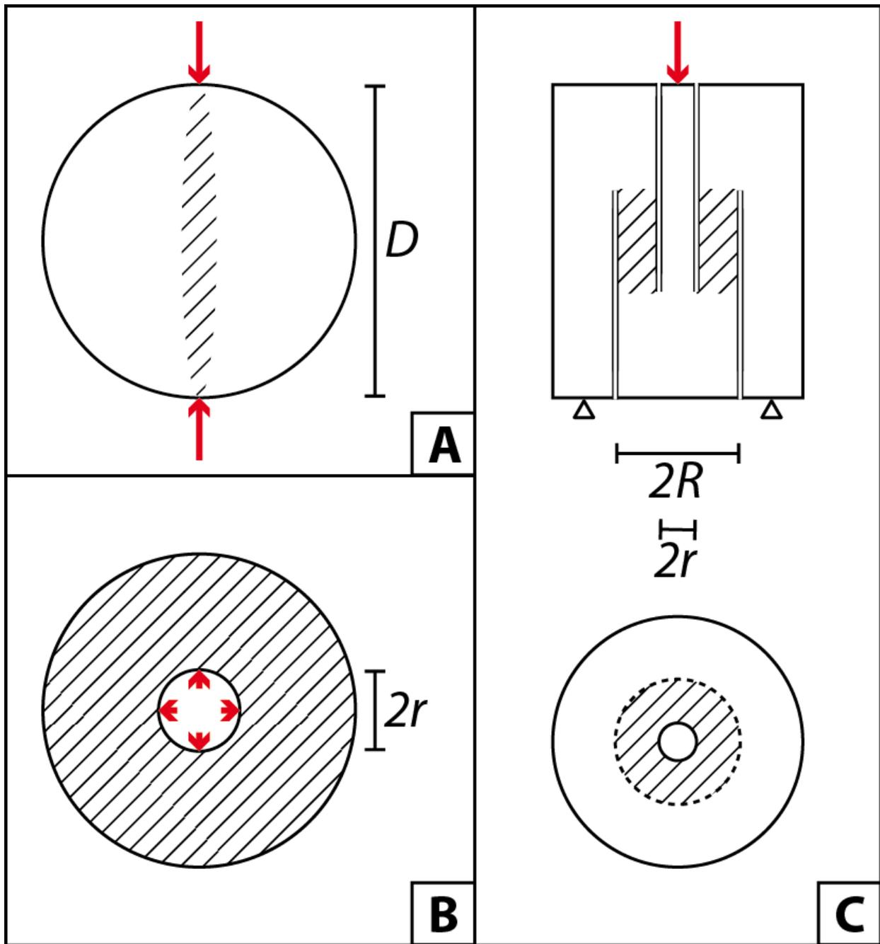
**Figure 1.** Sketches of the three tensile test methods. A: BDT side view, B: MF top view, C: MTT side view cross section (upper) and top view (lower).
