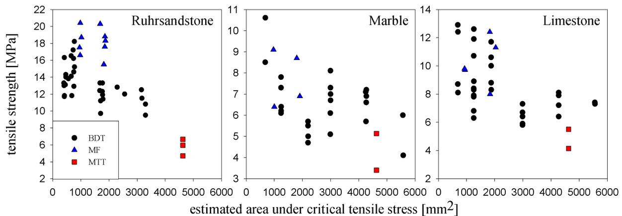
**Figure 6.** Tensile strength results plotted against the assumed area under tension. BDT: diameter x thickness, MF: surface area of the borehole and MTT: twice the surface area between the outer and inner borehole, upper and lower.
