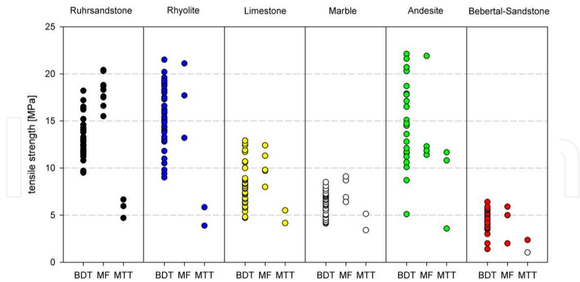
**Figure 3.** Results of all tensile strength test. BDT: Brazilian Disc Test, MF: Minifrac, MTT: Modified Tension Test. Hollow circle in Bebertal sandstone MTT tests represents two results of the highly eccentrical MTT tests.
