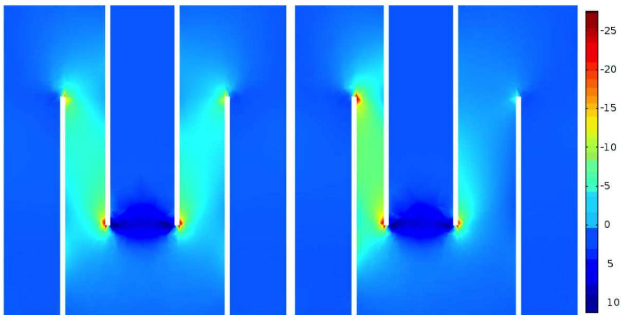
**Figure 5.** Slice through a linear elastic 3D FEM model of MTT tensile test. Values of axial stress are given in MPa where negative values stand for tensile stress. Left model represents a perfectly centralized sample. Right model shows the stress distribution for a eccentricity of 6 mm towards the left edge.
