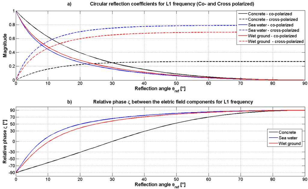
**Figure 3.** Co- and cross-polarized circular reflection coefficients for L1 (a); and relative phase change between the electric field components due to reflection process for L1 (b). For the exemplary material properties of concrete, sea water and wet ground.
