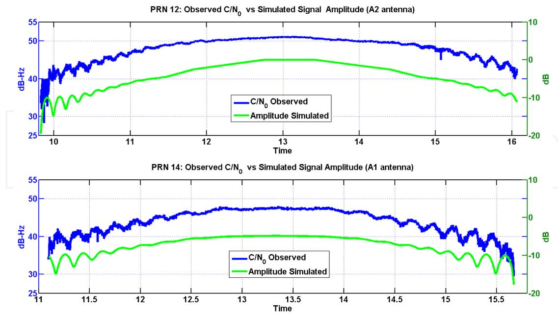
Figure 8. Observed C/N<sub>0</sub> values versus simulated signal amplitude for PRN 12 and 14 for antenna A1
