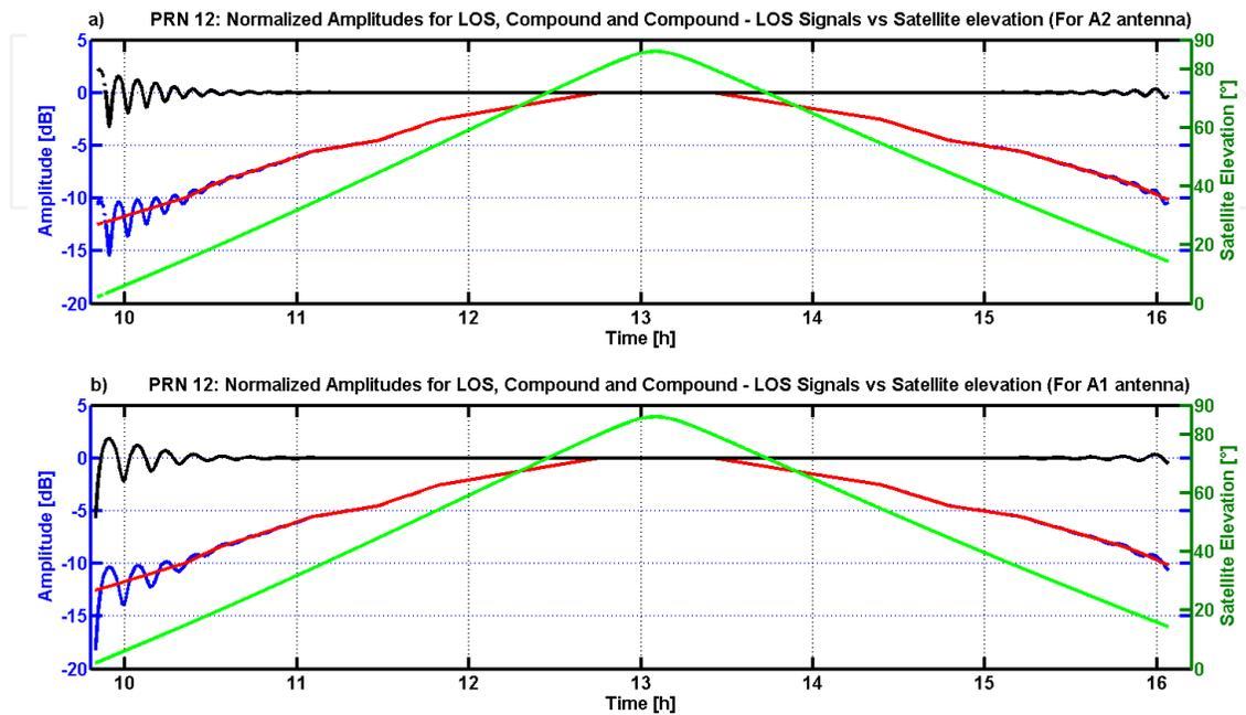
**Figure 6.** Simulated and normalized amplitude values versus satellite elevation for PRN 12 and reflector made of concrete. a) LOS, ground MPC and compound signal amplitudes for antenna position A2. b) LOS, ground MPC and compound signal amplitudes for the antenna position A1.
