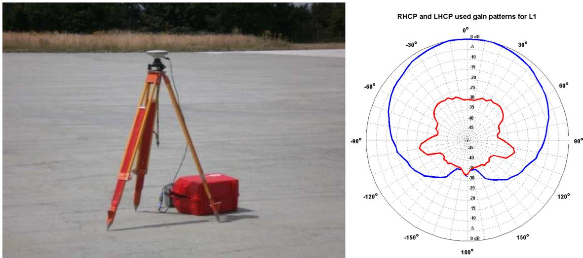
**Figure 5.** Left: Experimental set up of the Leica AX1202GG antenna. Right: The NOV702GG gain patterns [dB] for both orthogonal polarizations (RHCP in blue and LHCP in red) were used to model the antenna. Adopted from [77]
