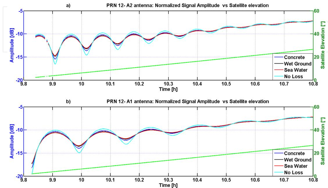
**Figure 7.** Normalized amplitude in [dB] of the compound signal for different material properties. Zoom at low elevation angles. (a): antenna A2, 2.053 m above the reflector, (b): antenna A1, 1.358 m above the reflector.
