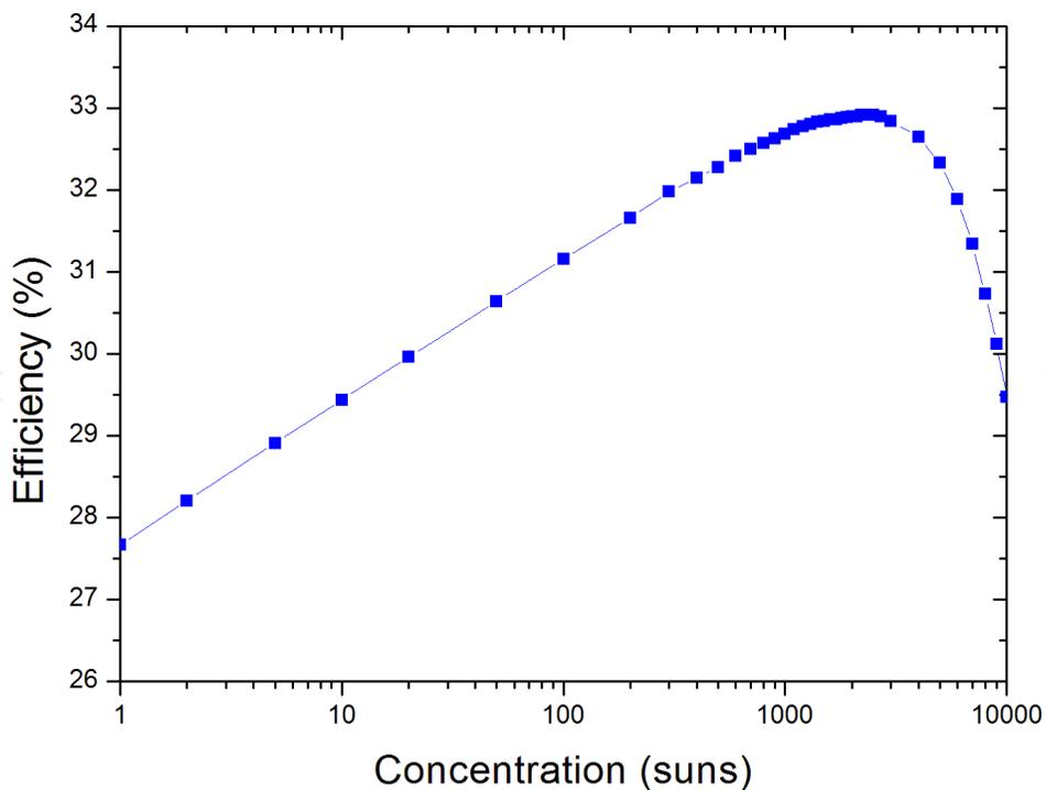
**Figure 7.** Simulation of the solar cell efficiency of a double-junction solar cell as a function of light concentration at a temperature of 320 K.
