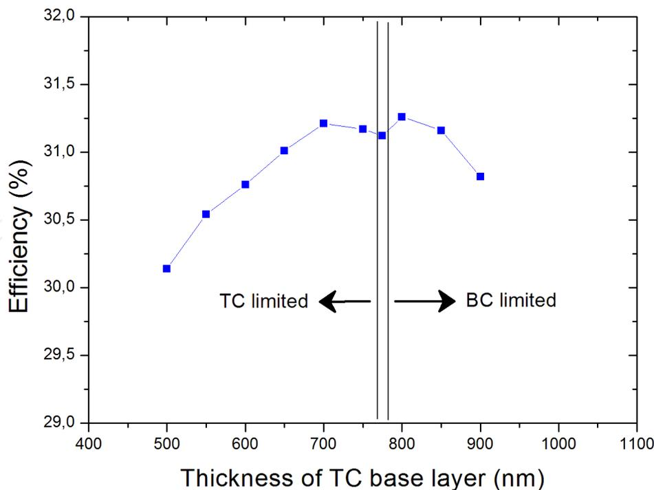
**Figure 12.** Simulation of the efficiency of a stand-alone double-junction solar cell as a function of top cell base thickness.
