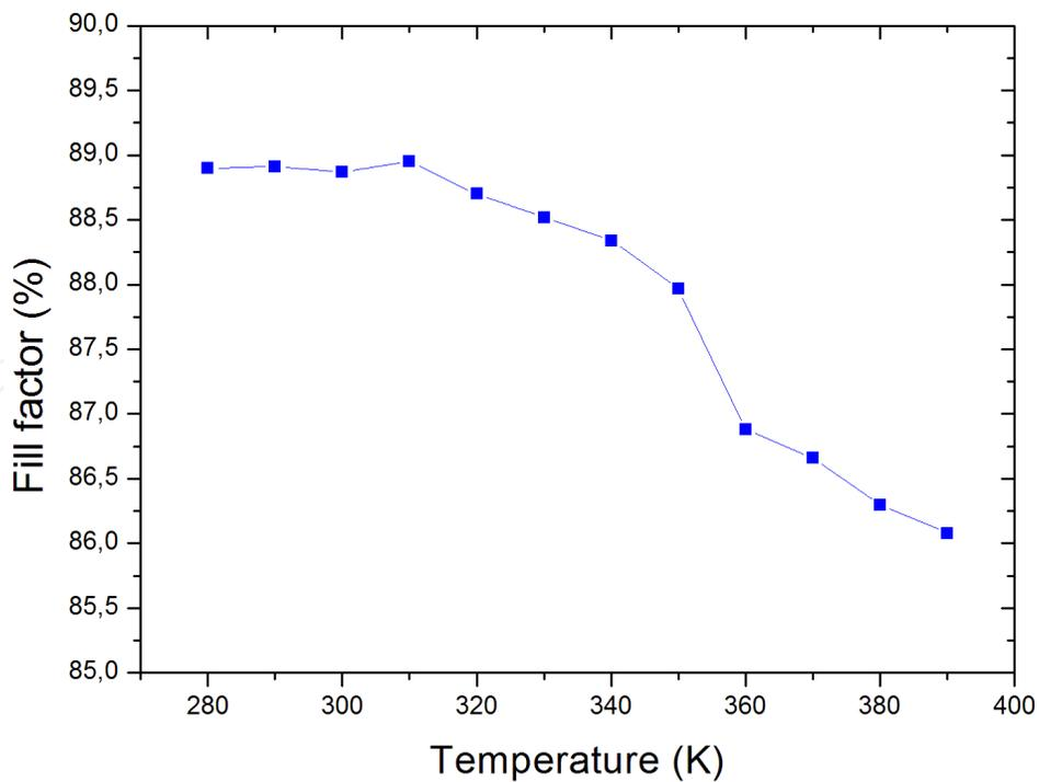
**Figure 5.** Simulation of the fill factor (FF) of a double-junction solar cell as a function of temperature at a concentration of 1000 suns.
