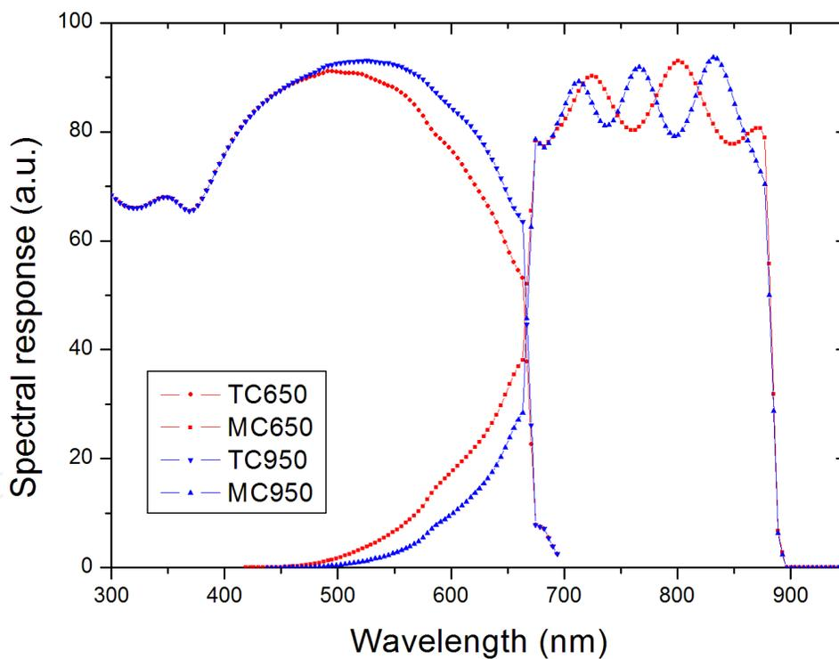
**Figure 14.** Simulation of the spectral response of a double-junction solar cell for two different TC base thicknesses (650 nm and 950 nm).
