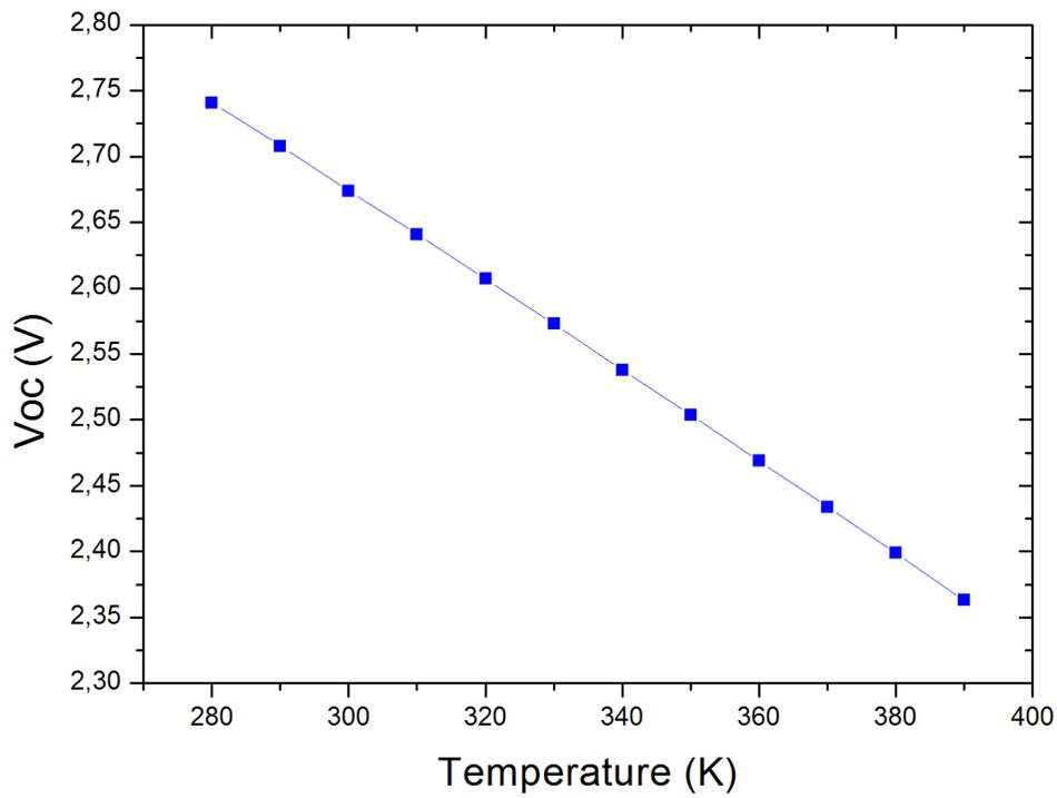
**Figure 4.** Simulation of the open-circuit Voltage ( $V_{oc}$ ) of a double-junction solar cell as a function of temperature at a concentration of 1000 suns.
