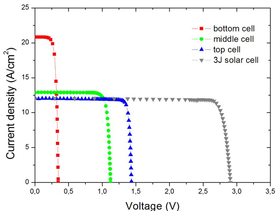
**Figure 8.** I-V curves of a triple-junction solar cell. There are given the three I-V curves of the subcells (top-cell, middle-cell and bottom cell) and the resulting I-V curve of the resulting 3J cell.
