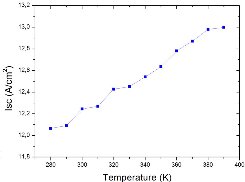
**Figure 3.** Simulation of the short-circuit current density ( $I_{sc}$ ) of a double-junction solar cell as a function of temperature at a concentration of 1000 suns.
