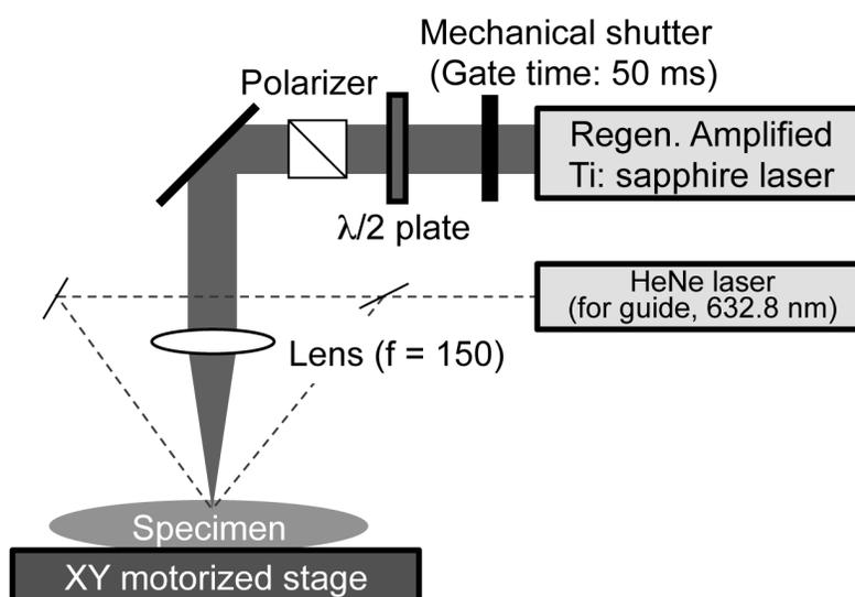
**Figure 1.** Experimental setup for femtosecond laser acupuncture.
