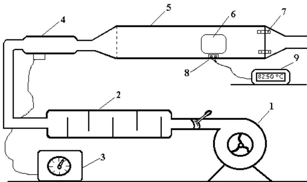
**Figure 1.** Experimental apparatus composed of: 1. fan; 2. molecular-sieve air dryer; 3. voltage regulator; 4. air heater; 5. wind tunnel; 6. observation port; 7. joint; 8. thermocouple socket; 9. thermocouple selector.
