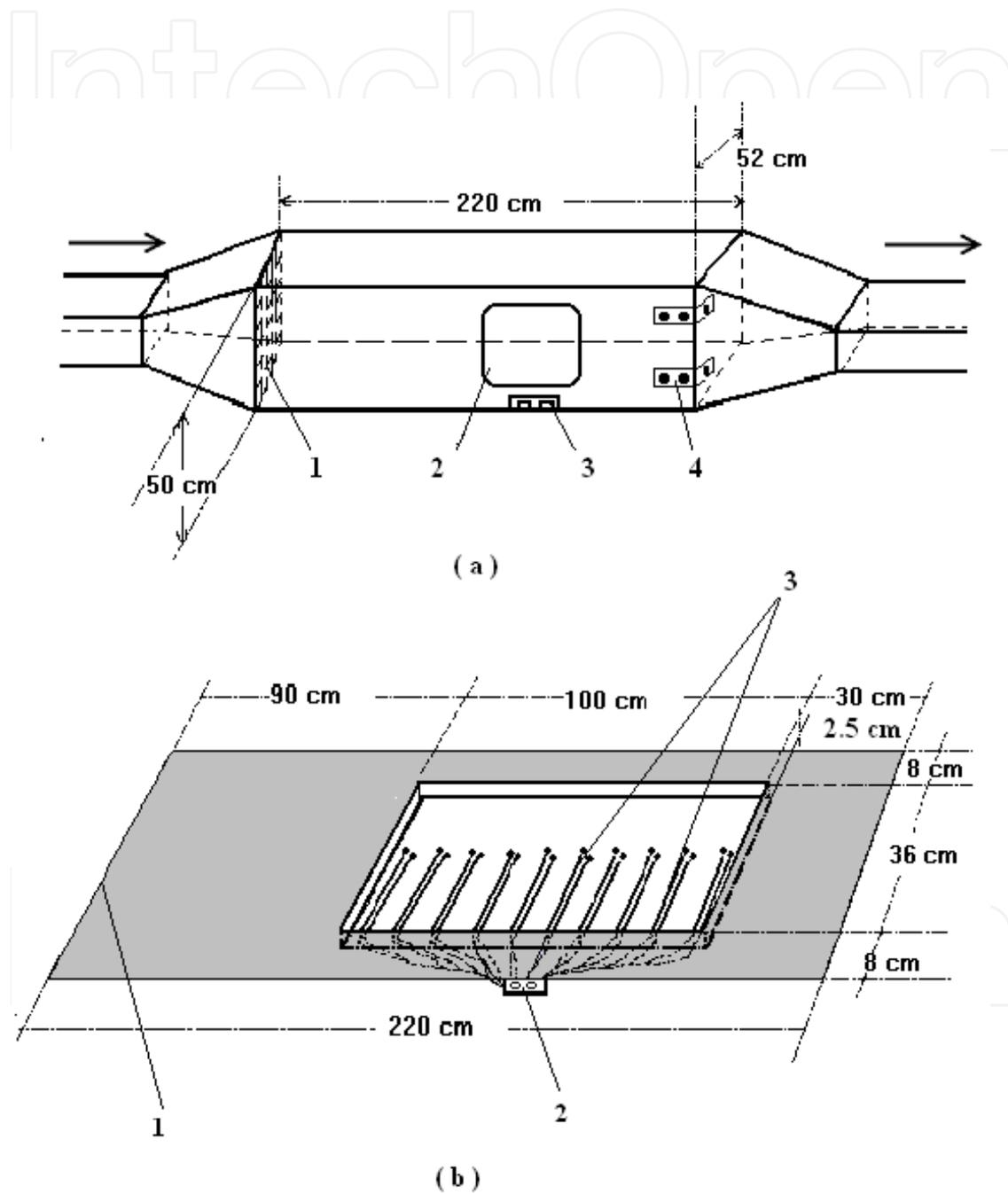
**Figure 2.** Details of (a) Wind tunnel: 1. smoothing grid; 2. observation port; 3.thermocouple socket; 4. joint, (b) Glass tray (clear) and flat plate (gray): 1. the leading edge; 2. thermocouple socket; 3. thermocouples.
