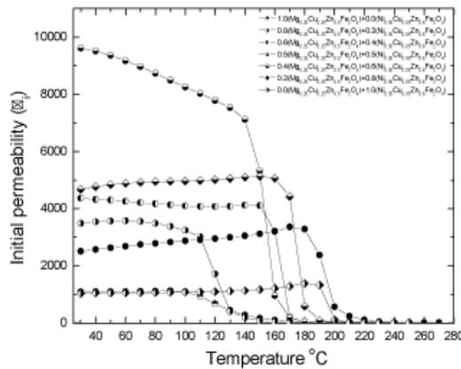
**Figure 5.** Variation of initial permeability ( $\mu_i$ ) with temperature at room temperature for the ferrite composites.
