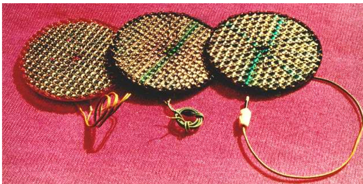
Figure 21. ITO-nSi portable sector-shaped solar modules fabricated by waste-free technology on 3 inch silicon wafers. Each module is assembled from 20 solar cells connected in serial.
