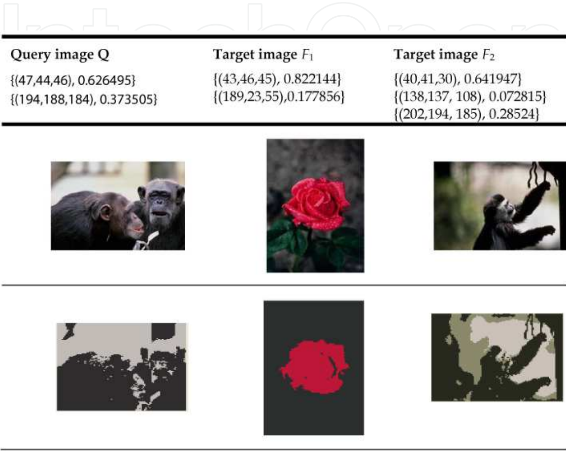
Figure 2. Example images with the dominant colors and their percentage values. First row: 3-D dominant color vector c_i and the percentage p_i for each dominant color. Middle row: the original images. Bottom row: the corresponding quantized images.
