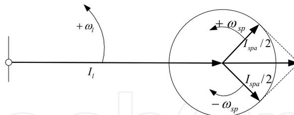
**Figure 1.** Vector representation of AM for broken bars
